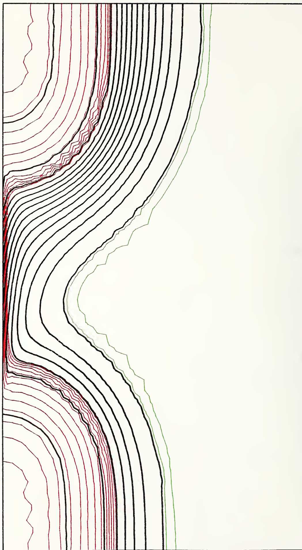
Figure 15. The potential, electron density, and hole density in the 1.83\text{--}\mu\text{m} transistor at a bias of V_g = 2.0\text{ V} and V_d = 2.0\text{ V} .
