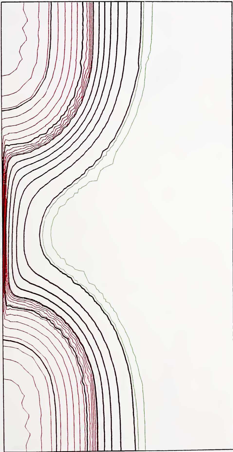
Figure 14. The potential, electron density, and hole density in the 1.83 - \mu\text{m} transistor at a bias of V_g = 2.0 V and V_d = 0.25 V.
