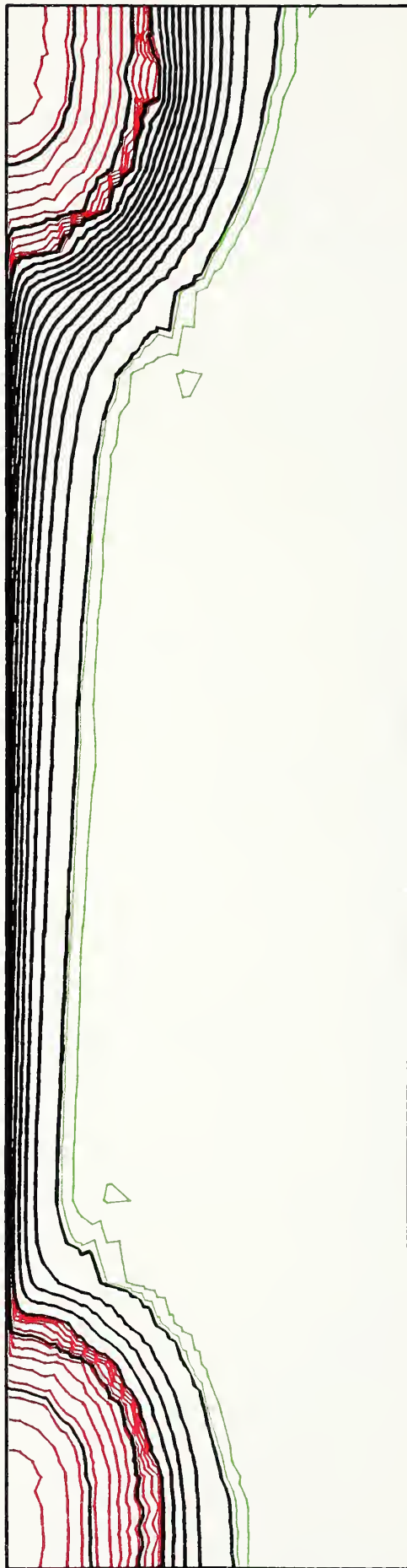
Figure 11. The potential, electron density, and hole density in the 8.17- \mu\text{m} transistor at a bias of V_g = 2.0\text{ V} and V_d = 2.0\text{ V} .
