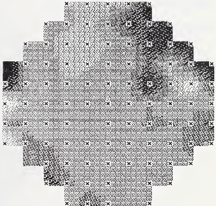
Figure D-11. Wafer map of n -channel calculated conduction factor, Device no. 3.
