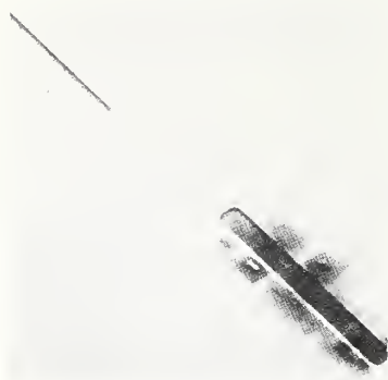
(a) Nominally 1 and 3- \mu\text{m} wide clear lines showing contamination buildup on 3- \mu\text{m} wide line; 2,000X.
