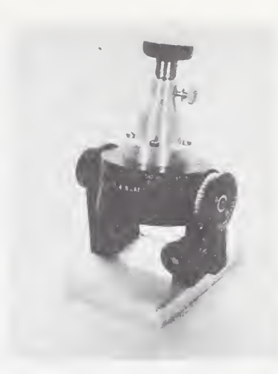
Figure 36. Two-axis, variable-angle substrate holder.
