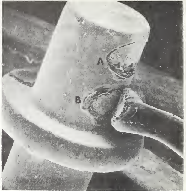
Figure 39. Scanning electron micrograph of the emitter post of a power transistor showing the imprint of a weak electrical discharge weld (A) that lifted off at low pull force and a partially peeled back 300- \mu\text{m} (0.012-in.) diameter aluminum wire bond (B). (Magnification: \sim 36\times ).
