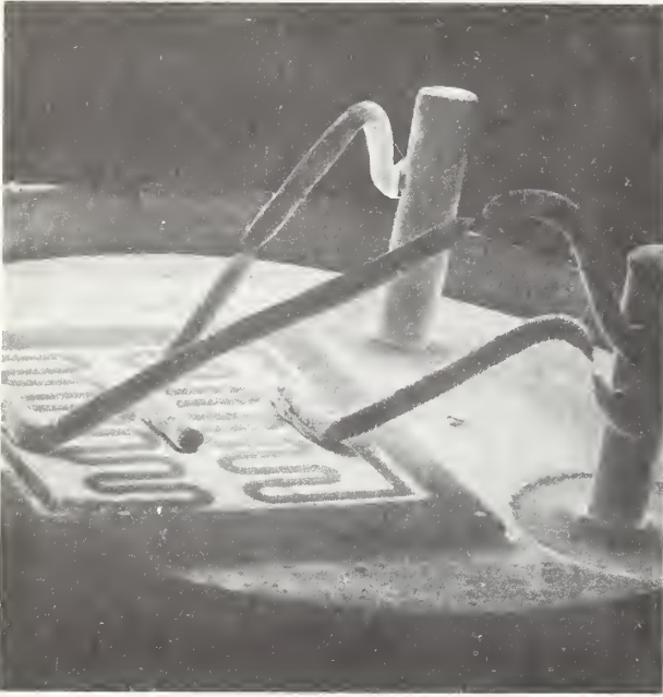
Figure 38. Scanning electron micrograph showing the typical failure mode of well-made, 200- \mu\text{m} (0.008-in.) diameter, aluminum wire bonds subjected to a destructive double-bond pull test. (For clarity, the wires were carefully bent back into their approximate positions at rupture. Magnification: \sim 13\times ).
