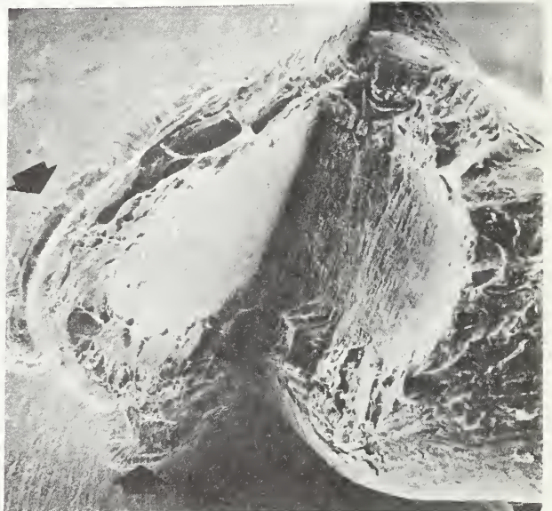
Figure 41. Scanning electron micrograph of the lower emitter post bond of figure 39 at greater magnification to show absence of deformation or welding in the center region of the bond and purple plague regions (arrows) around the outer perimeter of the weld. (Magnification: \sim 130\times ).
