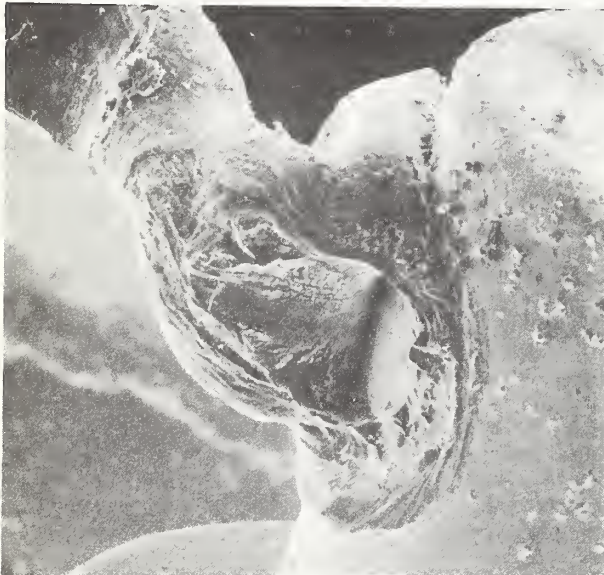
Figure 40. Scanning electron micrograph of a partially lifted, very strong electrical discharge weld to a gold-plated post showing the absence of welding in the center of the bond. (Magnification: \sim 72\times ).
