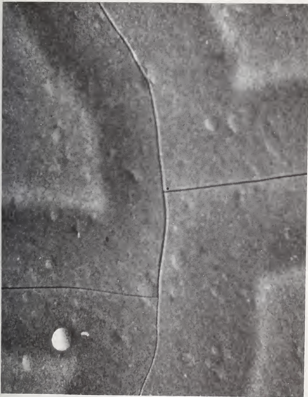
Figure 12. Glass microcracks in sample shown in figures 8, 10 and 11 as observed by SEM at 4800X and 30° from the perpendicular. Width of crack from this high-magnification photograph is approximately 0.2 \mu\text{m} .
