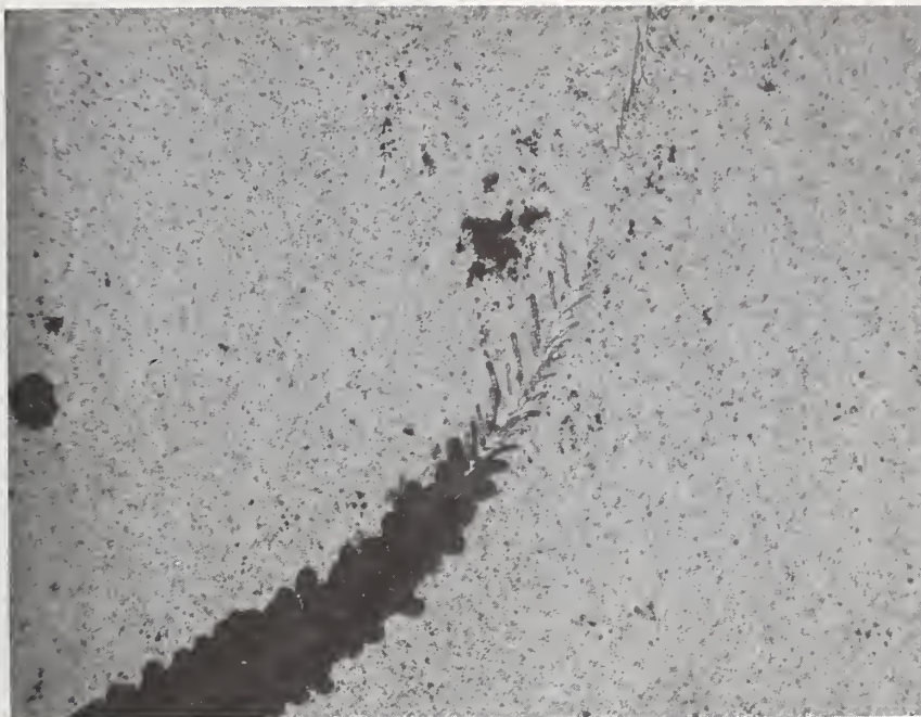
Figure 3. Scratch-induced heavy damage in glass layer made visible by 20-min aluminum etching. Scribe direction was apparently downward with increasing pressure. Sample structure as noted in figure 1 (385X, brightfield).
