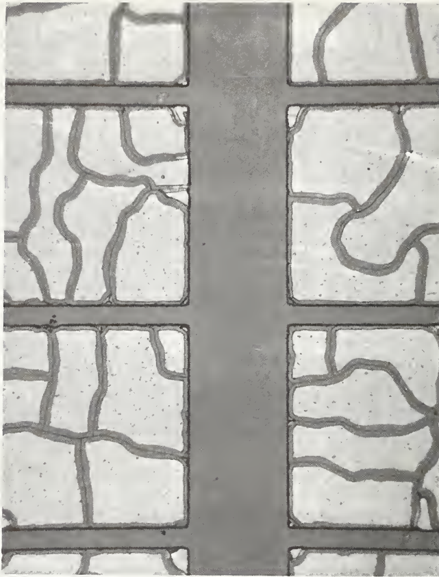
Figure 8. Optical photomicrograph of stress cracks of a CVD silicon dioxide film of 1- \mu\text{m} thickness deposited over oxidized silicon with squares of 105 x 105 \mu\text{m} of evaporated aluminum. Demarcation was achieved by 10-min aluminum etching. Cracks surround most of pattern along edge of aluminum. Differences in the width of the inside area are most probably caused by differences in the width of the cracks (150X, brightfield).
