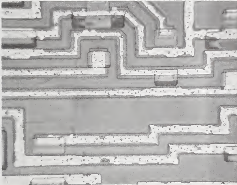
Figure 18. Developed thin edge coverage of PSG over edges of aluminum interconnect of an IC. The aluminum line edges became exposed in many places after 50% of the glass coating was removed by selective etching (385X, brightfield).
