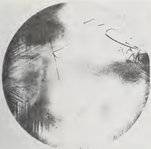
Figure 52. X-ray topograph of a 63-mm diameter silicon wafer containing process-induced defects.
