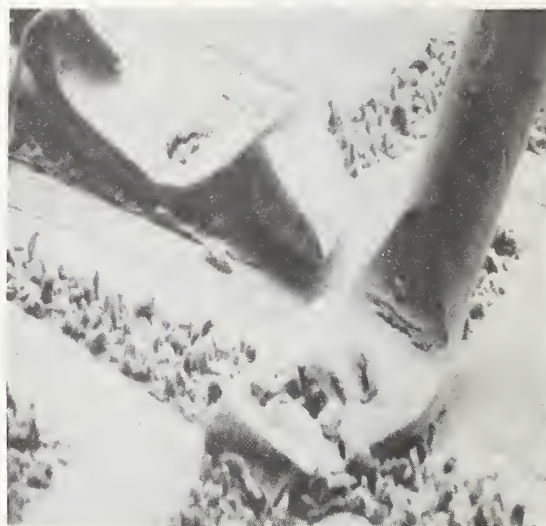
c. Large bond deformation \sim 2.2 times wire diameter as determined from head-on SEM photomicrograph. Magnification \sim 230\times .
