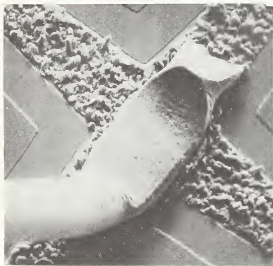
b. Average bond deformation \sim 1.6 times wire diameter as determined from head-on SEM photomicrograph. Magnification \sim 460\times .
