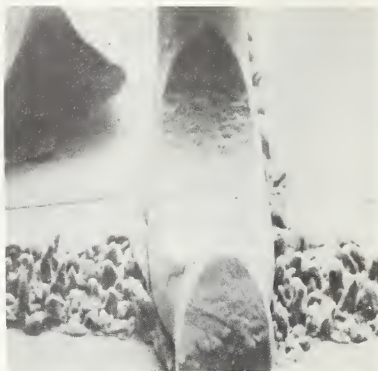
a. Small bond deformation \sim 1.2 times wire diameter. Magnification \sim 585\times .
