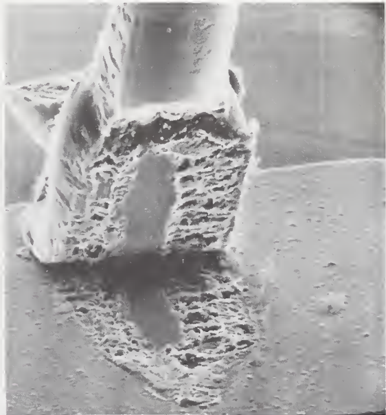
Fig. 3-15. SEM photomicrograph of the lift-off pattern of a partially removed bond made under laboratory conditions. A similar pattern can be observed on both the wire and the pad. Again the center portion of the bonded region is not welded. Magnification: 900 x.
