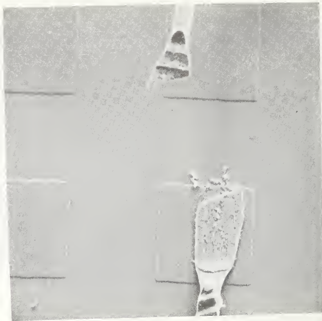
a. Severance of wire by heel of tool. Magnification: 200 x.
