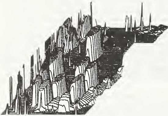
Figure 42. ASLEEP scan of 30-mil (0.76-mm) diameter MOS capacitors on 35-mil (0.89-mm) centers.
