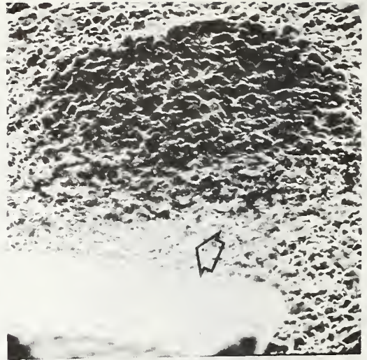
a. Depression in the substrate remaining after beam was peeled back. The arrow denotes the largest broken welded area. Magnification: \sim 580\times .)
