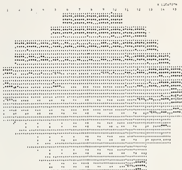
Figure 18. Map of threshold voltage where the magnitude of threshold voltage is indicated by the darkness of the position characters.
