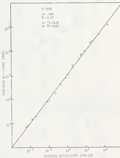
Figure 3. P-Type Calibration Curve - Spreading Resistance vs. Resistivity.
