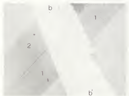
Figure 14 Double exposure photograph of wire images and sample's bevel surface. Images have completely crossed and are positioned edge to edge. This is the final step of measurement. Orientation is 44^{\circ} . Total \alpha = 1/2 \times 47^{\circ} = 23.5^{\circ} . Specimen bevel angle = 69.5' where s = 0.0153 in. and d = 0.0805 in.
