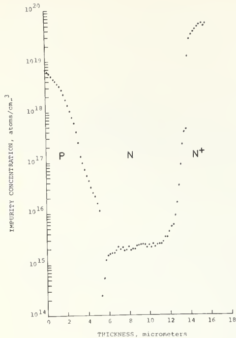
Figure 8. Boron Diffusion into an N-type Epitaxial Layer on an N + Substrate-Impurity concentration vs. Thickness.
