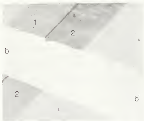
Figure 11 Photograph taken with MSAM system showing double images (1 & 2) of wire. Images are positioned edge to edge at this orientation of sample stage: 91^{\circ} . This is the starting point of specimen bevel angle measurement. By a second exposure, image (b-b') of sample's bevel surface is also shown. NOTE: microscope focal point must be changed between these exposures.
