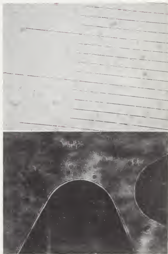
Figure 7. Shadow graph of two spreading resistance probe tips with a 10 \mu\text{m} stage micrometer scale.
