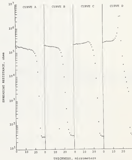
Figure 6. Effect of Time Delayed Dopant Injection on the Interface Between an N + Substrate and an N-type Epitaxial Layer.
