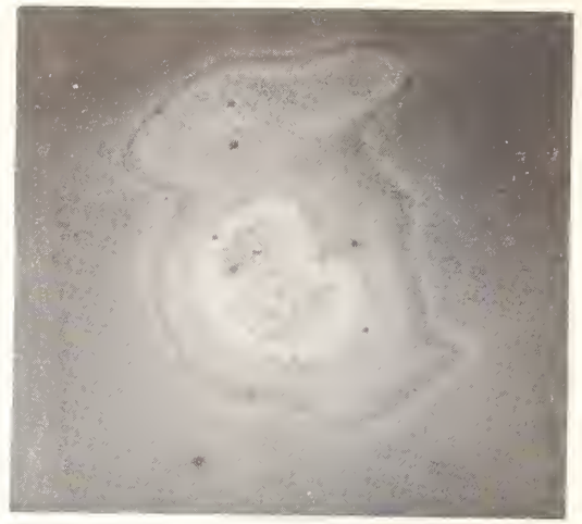
Figure 10. Same area as Figure 9, at higher magnification, showing damage to substrate at center, 416 J/cm 2 (230X).
