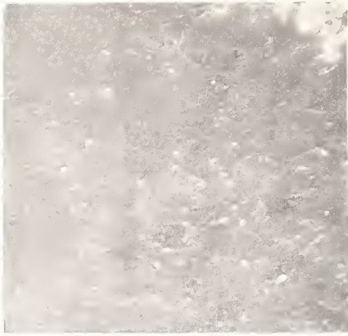
Figure 8. Detail of most heavily damaged part of Figure 6, showing partial removal of coating by blister formation and bursting, 233 J/cm 2 (1000X).
