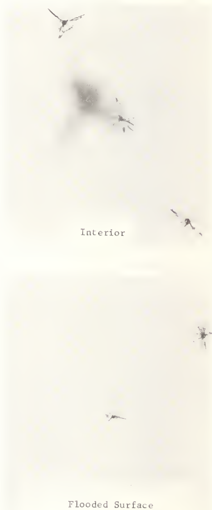
Figure 2. Photo micrographs of 1.06 \mu\text{m} laser damage sites in fused silica.
