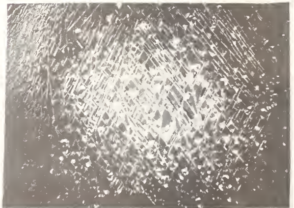
Figure 6b. KCl. One shot at 17 \text{ J/cm}^2 in 75 nsec. Damage with breakdown.
