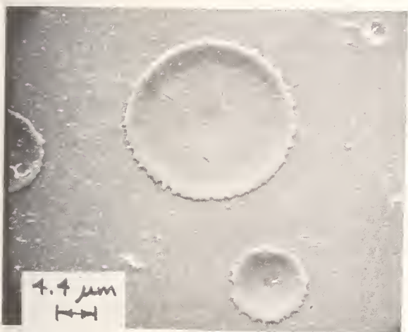
Figure 25. A close-up view of the craters shown in figure 24. The cracks were neatly formed according to some crystallographic orientation.
