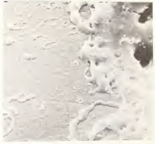
Figure 27. Detail of interface between melted area and undisturbed film shown in Figure 24. \text{MgF}_2/\text{MgO}/\text{CaF}_2 , 114.5 \text{ J/cm}^2 (5900X).
