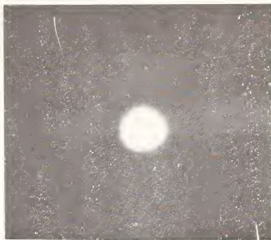
Figure 2. 200 micron plasma detected by microscope. Note the unambiguity of the presence of the plasma. The specks on photo result from dirt on the original photo.
