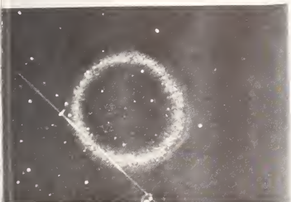
Figure 2a. Single crystal germanium, 20 \Omega \times \text{cm} , n-type. One shot at 17 \text{ J/cm}^2 in 75 nsec. Magnification is \times 50 .
