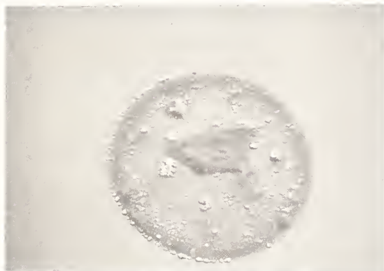
Figure 20. SEM photograph of a damage site on a single quarter-wave thick film of \text{TiO}_2 (sample 0121) where a spark was detected. The site dimension is 110 microns, from left to right.
