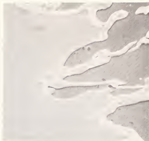
Figure 22. Detail of edge of damaged area (Figure 21) of evaporated gold film on beryllium copper substrate. 347 \text{ J/cm}^2 (2100X).
