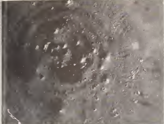
Figure 10. Optical micrograph taken using Nomarski lens. Note interference rings within the damage. Photo shows 1.1 mm width.
