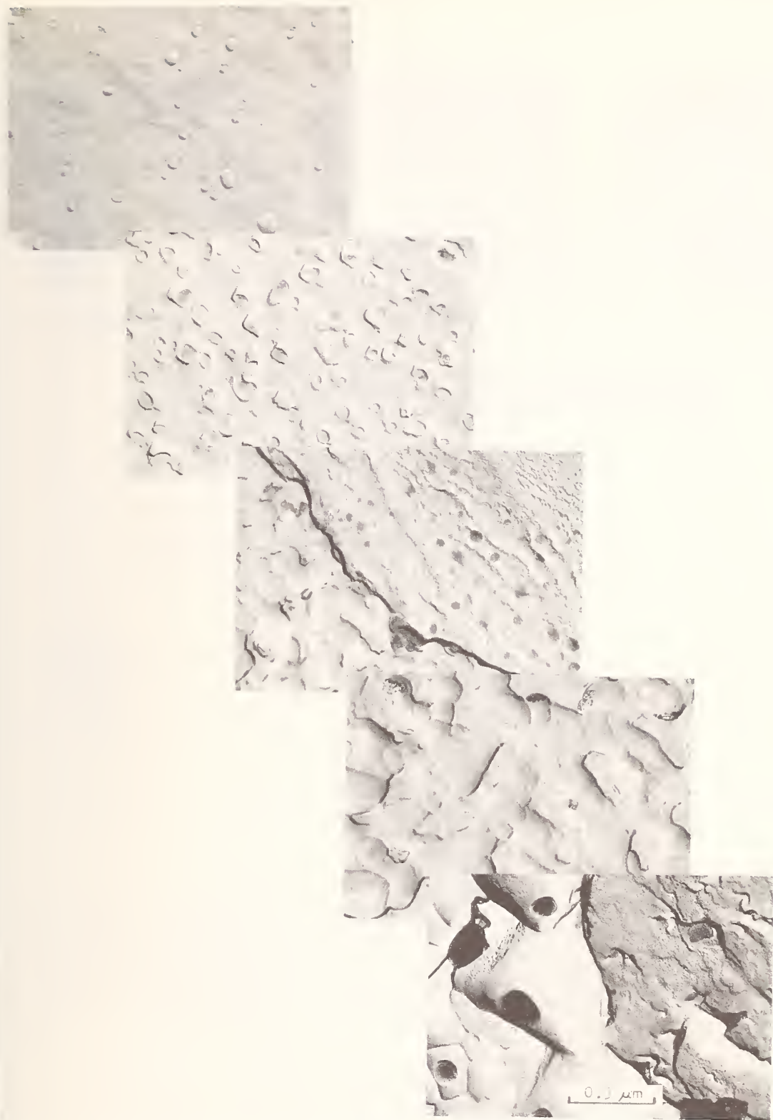
Figure 9. Electron micrographs illustrating the damage morphology of ALQLOY from the center outward edge of damaged area.
