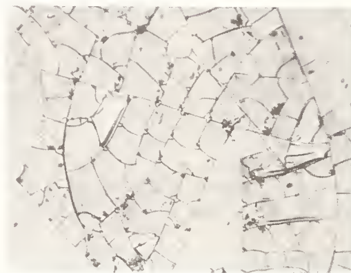
Figure 9. Plasma induced thermal cracking on glass. Area in photo is 0.6 mm wide.
