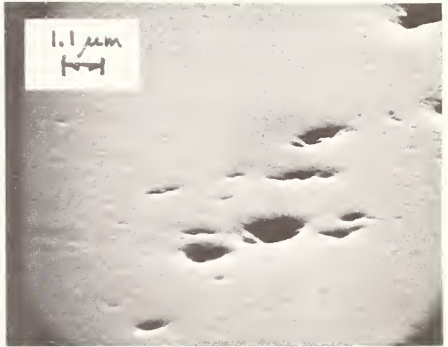
Figure 7. SEM photograph of defects of a group of holes on a single quarter-wave MgF_2 film.
