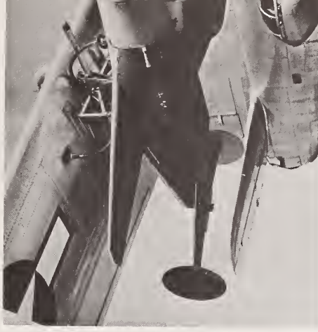
The Bureau helped develop the Bat, the first guided missile ever used in combat. It was unpowered, gliding from the release plane to the target.
