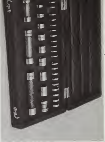
Using a technique invented by William E. Hoke, the Bureau produced 50 precision sets of gauge blocks for use by American industry during the first World War.
