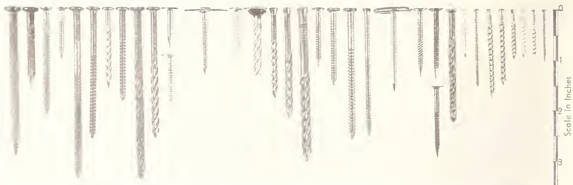
Fig. 1 The 33 nails and 2 alternative nails used for the erection of the V.P.I. Demonstration House during 1955.
