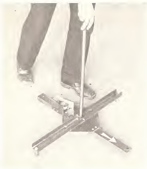
Fig. 1. "Measuring chair" for measuring flatness of floors with reference to square furniture with 0.5 m (0.55 yd) side. The crossing arms form diagonals in the square. At the ends of the arms there are three fixed legs, the fourth being vertically adjustable. This is connected with a dial from which the deviation of the floor from the plane can be directly read off.
