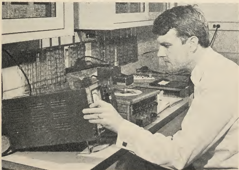
The color density of a radiochromic dye film is measured after electron irradiation. Density variations indicate changes in the dose distribution of the electron beam.
