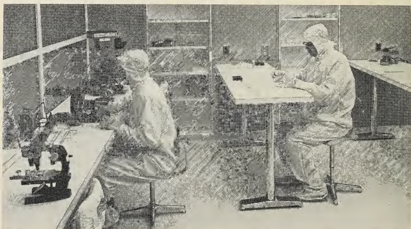
Standard reference materials being prepared by the dispersal of chemically loaded ion-exchange beads on glass slides in a clean room.
