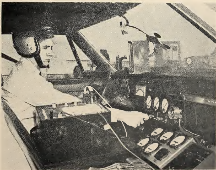
Instrumented test vehicle used for evaluation of braking systems under normal and various types of failure conditions.
