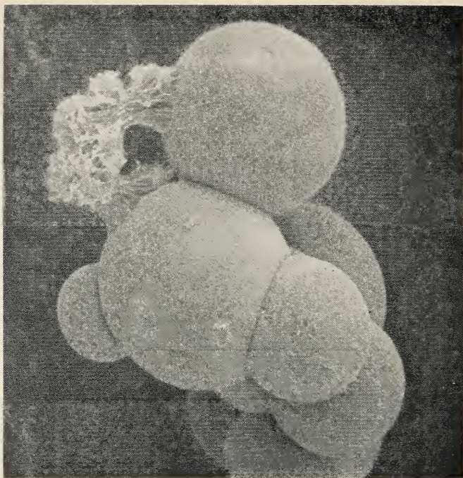
66-Nylon is being studied to determine the manner in which the chain molecules fold during crystallization. Shown here is a scanning electron micrograph of (X520) spherulites and other aggregates (top left) of 66-Nylon grown from a concentrated solution of the polymer in glycerol.
