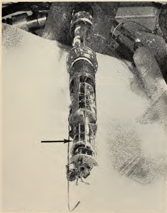
He 3 -He 4 dilution refrigerator produces temperatures below 0.1 K. Refrigeration is produced in a chamber inside a coil (arrow) used to measure the temperature. Suspended from the chamber are two devices to be tested—a Josephson-junction thermometer on the disc and a heat exchanger to the left. In use the refrigerator is surrounded by a vacuum space and several thermal shields.
