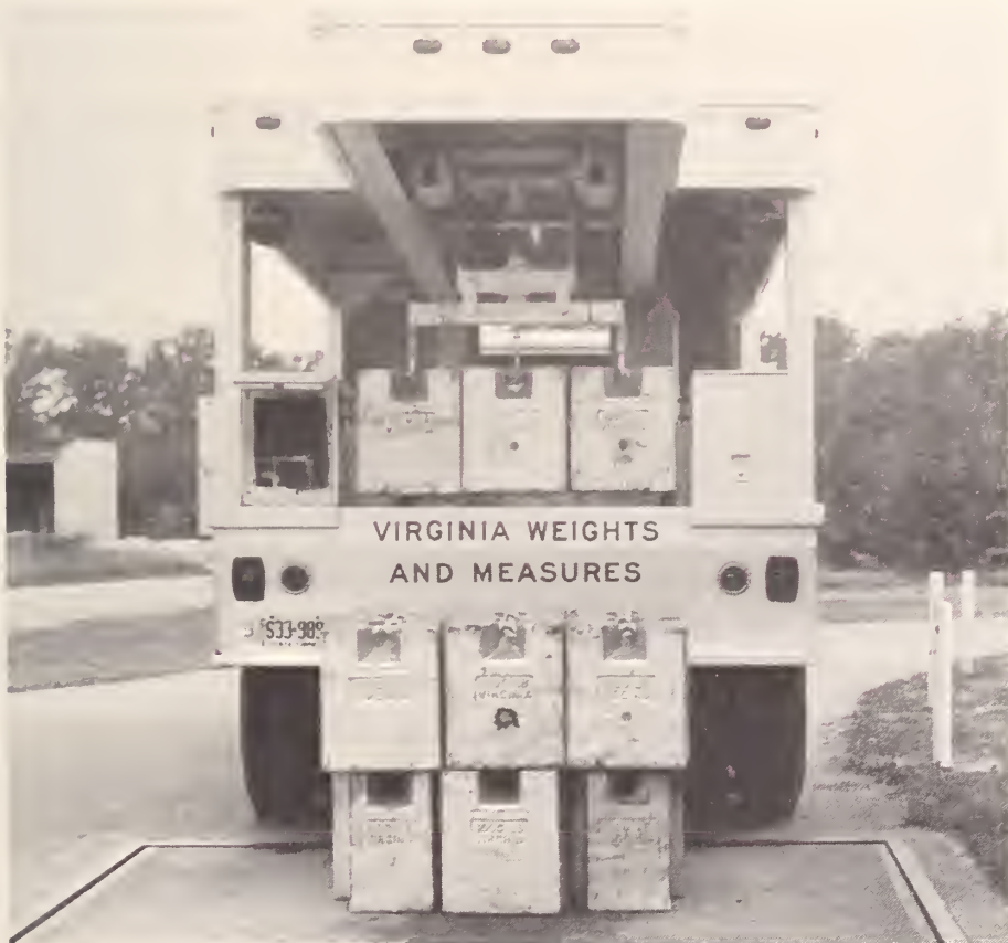
FIGURE 2.— Rear of Virginia unit showing test load.
