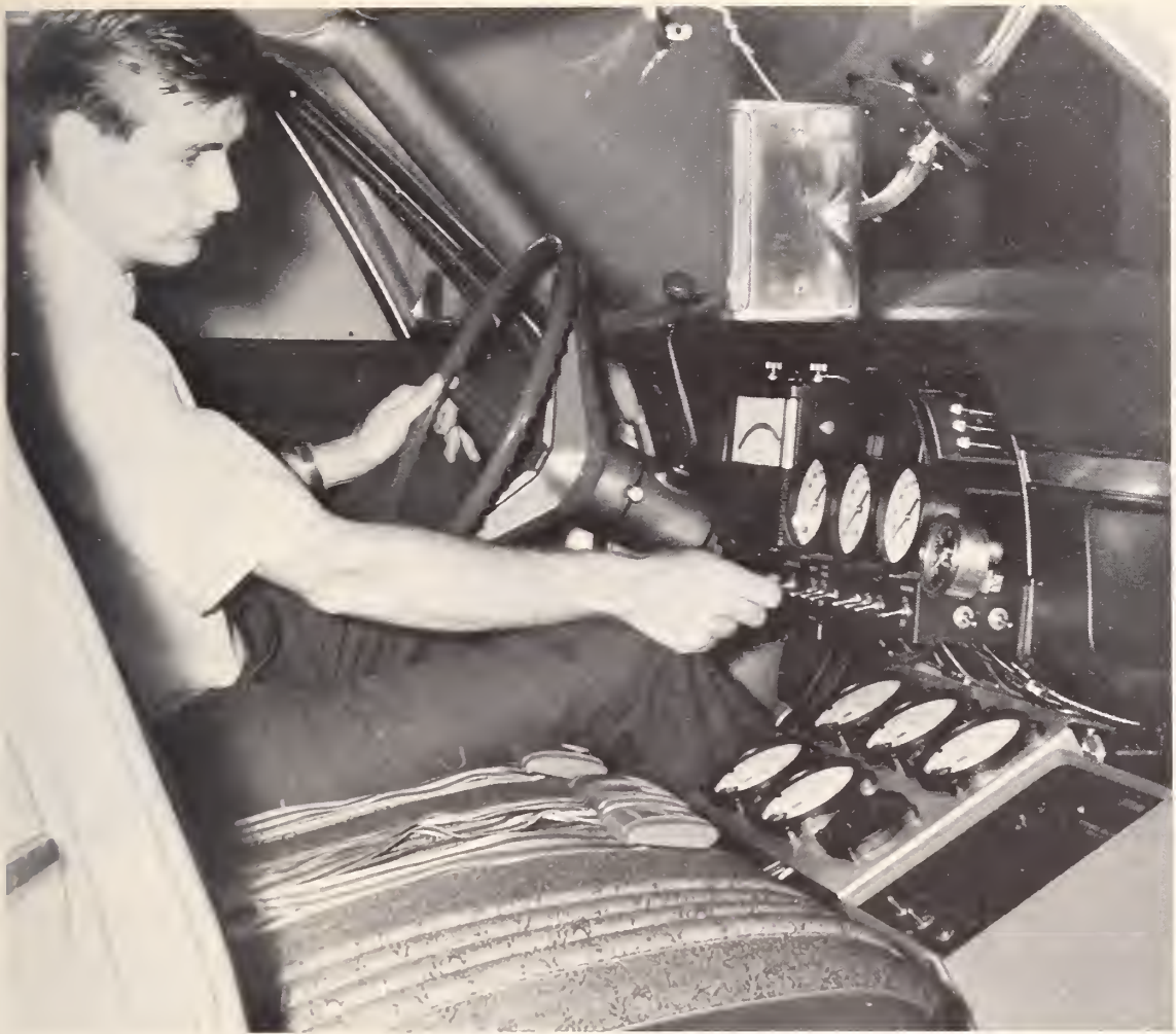
FIGURE 2.—Interior of instrumented vehicle for brake system testing.
