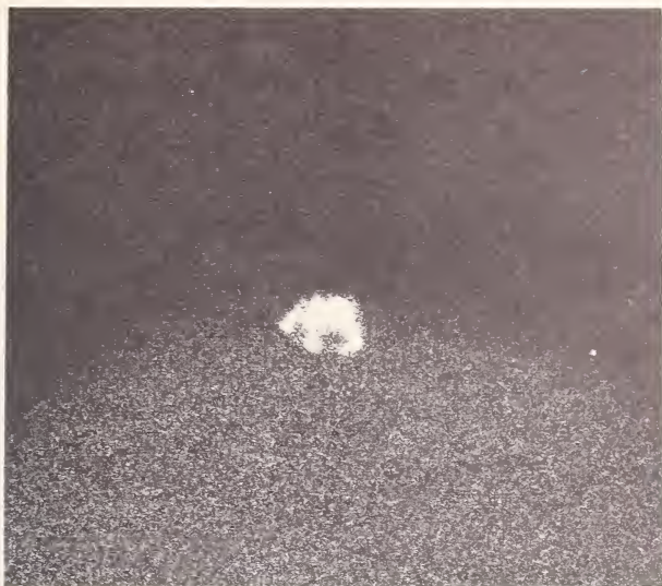
Figure 3. Autoradiograph of a disc from a zone refined monocrystalline silicon rod containing mercury.
