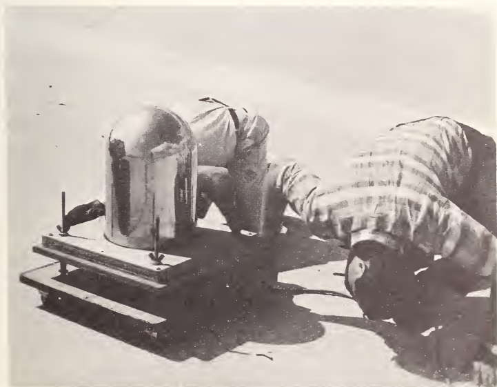
Figure 3. Positioning of portable 14 MeV neutron generator in field fast neutron activation analysis.
