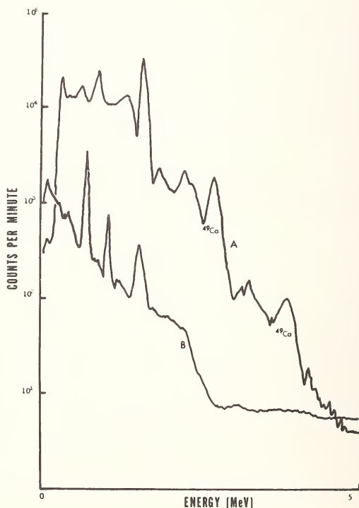
Figure 1. Gamma spectra of (n,\gamma) thermal neutron products in concrete for 10 seconds at 8 \times 10^{12} \text{ n}\cdot\text{cm}^{-2}\cdot\text{sec}^{-1} . Curve A—9 min decay; Curve B—8.5 h decay.
