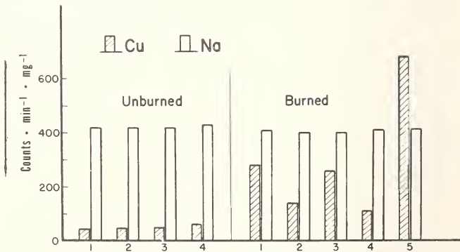
Figure 6. Copper and sodium activities of irradiated skin specimens.
