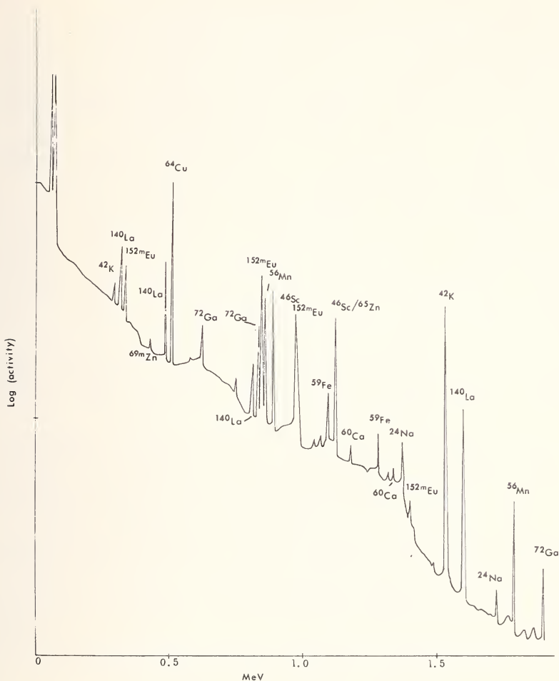
Figure 2. Ge(Li) spectrum of W-1 after ^{24}\text{Na} separation.
