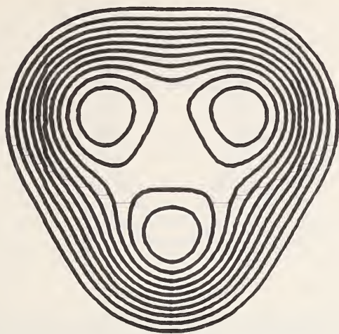
FIGURE 8. Scattering density in a plane perpendicular to the three-fold axis of ammonium fluorosilicate. The hydrogen atoms should lie approximately in this plane. This experimental result may be understood either in terms of the static disorder suggested by figure 7 or by a more dynamic situation.
