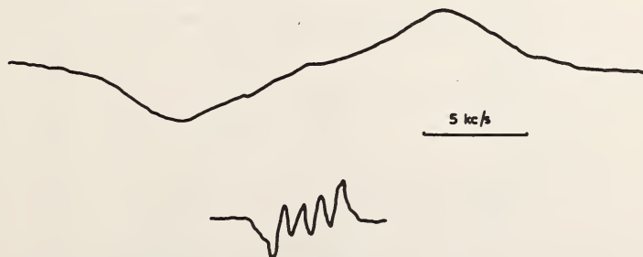
FIGURE 6. A spin-spin multiplet resolved in the n.m.r. spectrum of a solid by the technique of rapid specimen rotation [35]. The upper trace is the ^{19}\text{F} n.m.r. derivative spectrum of a static specimen of polycrystalline hexafluoroarsenate, \text{KAsF}_6 . The lower trace is the spectrum for the specimen rotated about the magic axis at 5.5 kHz displaying a quartet structure due to electron-coupled interaction between ^{19}\text{F} and ^{75}\text{As} nuclei.
