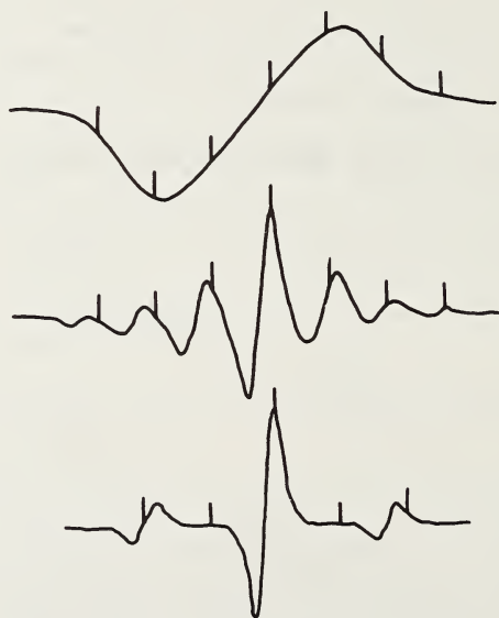
FIGURE 5. The effect of rapid rotation on the n.m.r. spectra of a solid [28]. Top: ^{23}\text{Na} n.m.r. derivative spectrum of a sodium chloride crystal at rest. Middle: spectrum for the same crystal rotated at 800 Hz about the magic axis. Bottom: spectrum for the crystal rotated at 1600 Hz about the magic axis. The markers are 800 Hz apart.
