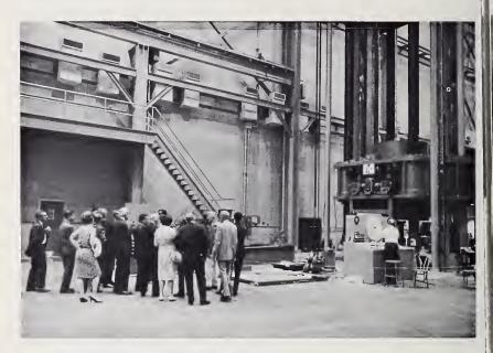
The above group is looking at the twelve-million-lbf capacity hydraulic testing machine, believed to be the world's largest, is being installed in the new NBS Engineering Mechanics Building. A unique facility, the machine will provide the force to calibrate multi-million-lbf capacity force-measuring devices for space and industrial applications and to test full-scale structural components. The machine has a total height of 101 ft, including 21 ft in a pit.
