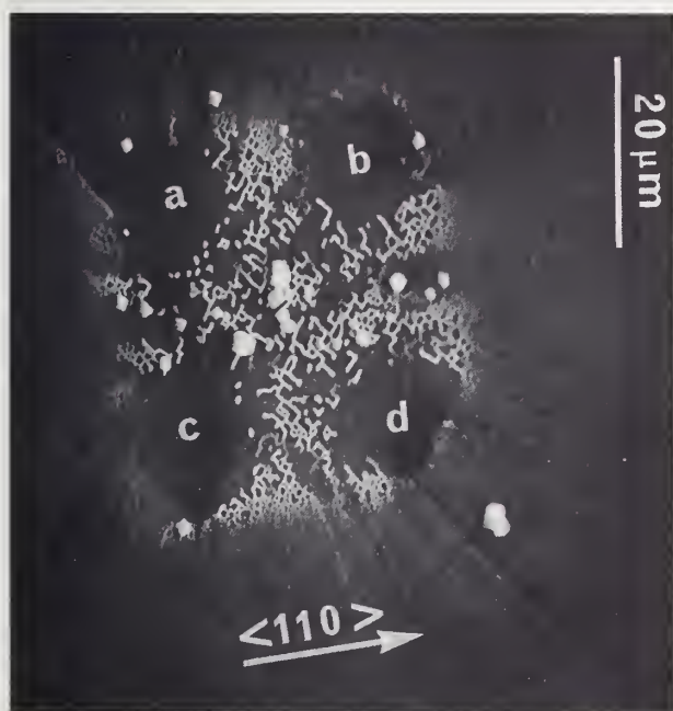
FIGURE 5. Scanning electron micrograph of a lenticular cavity showing development of lobes. (a, b, c, d).
