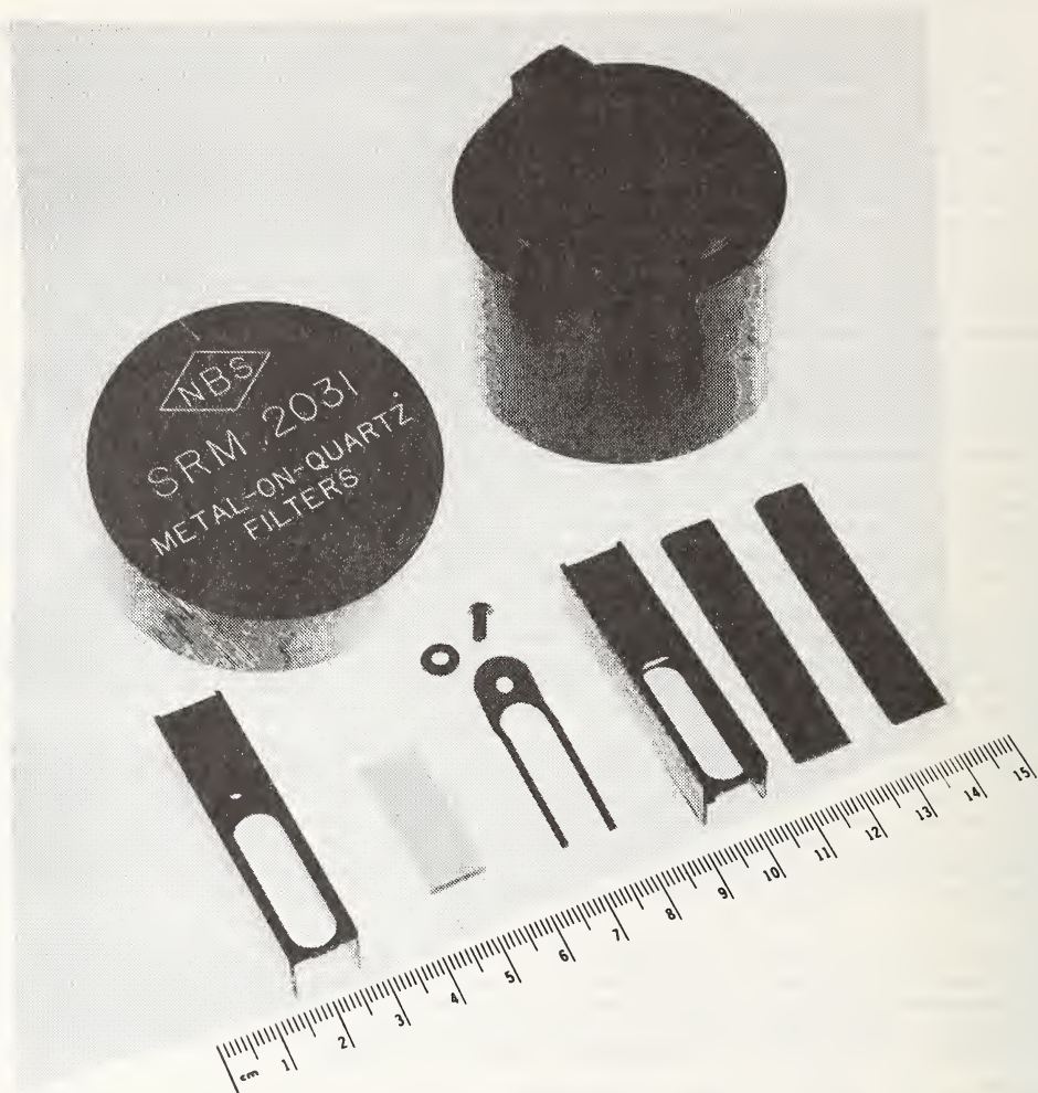
Top: Cylindrical container with its screw cap, both made of black-anodized aluminum alloy. Four filter holders can be stored in the cylindrical container. Bottom (from left to right): Aluminum alloy filter holder, 12.5 mm square and 58 mm high; Metal-on-quartz filter; Retaining spring of beryllium-copper with nylon screw and washer; Assembled unit; and two Delrin shutters. All metal and plastic parts are flat black.
