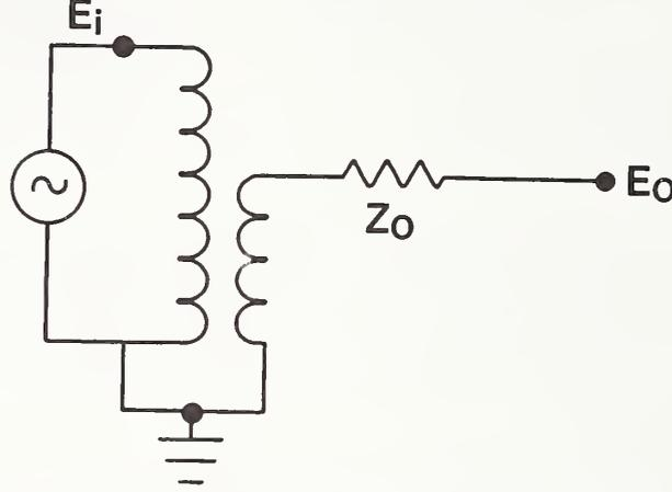
Figure 9. Equivalent circuit of a voltage transformer.
