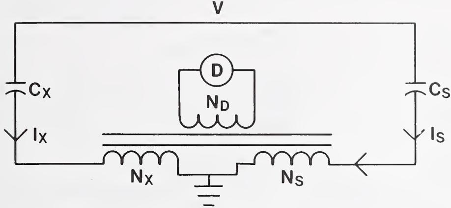
Figure 12. Basic current comparator bridge.
