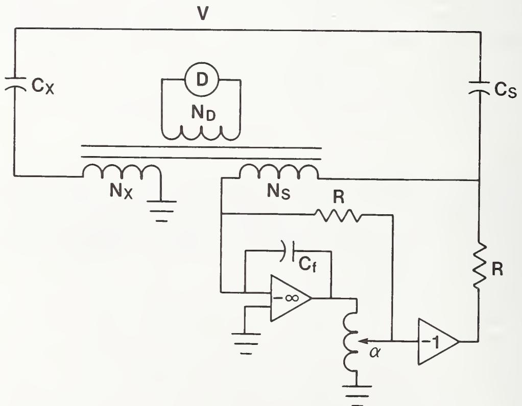
Figure 14. Current comparator with superior in-phase current balance.
