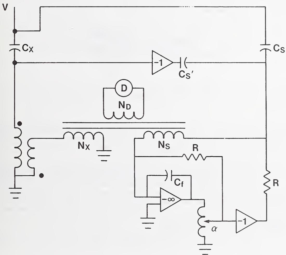
Figure 16. Current comparator bridge with external range extender.
