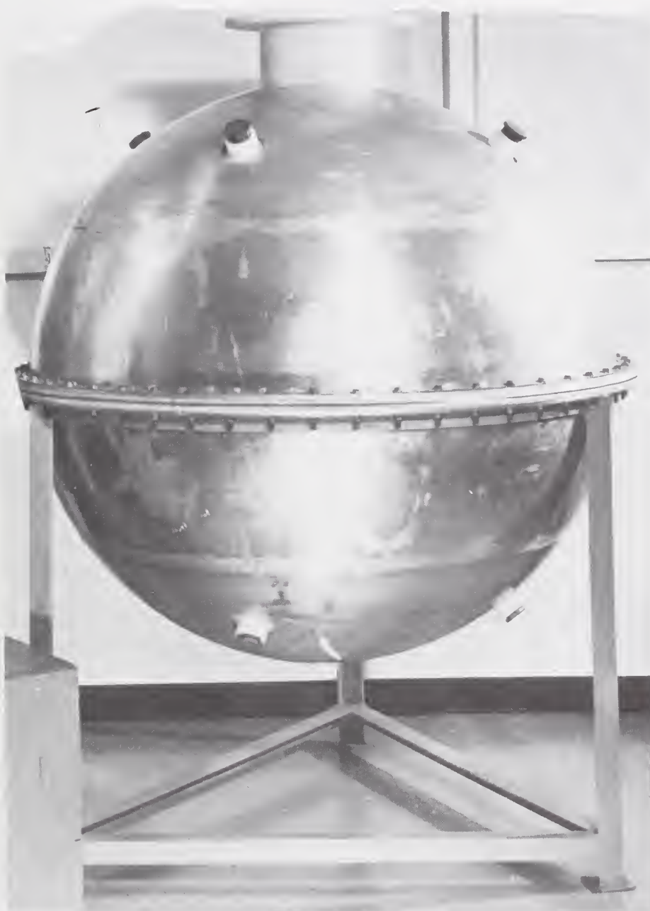
FIG. 3. A photograph of the aluminum shell which supports the polyethylene liner and \text{MnSO}_4 solution. Sources are pulled into the center of the solution by a Teflon can attached to a rope on a pulley, above, and a short steel bar at the bottom of the inside of the spherical tank.
