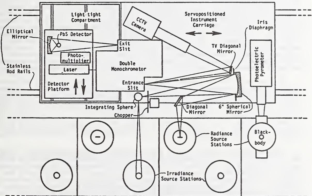
Figure 1. OPTICAL ARRANGEMENT OF FASCAL SYSTEM
