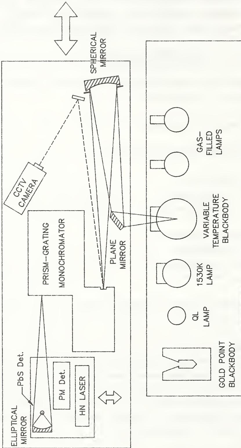
FIGURE 1. Spectral Radiance Measurement Apparatus
