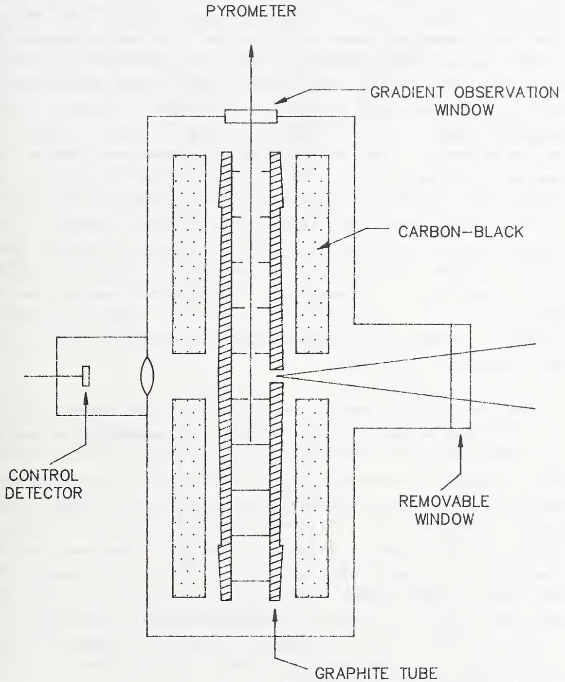
FIGURE 2. Variable Temperature Blackbody Schematic
