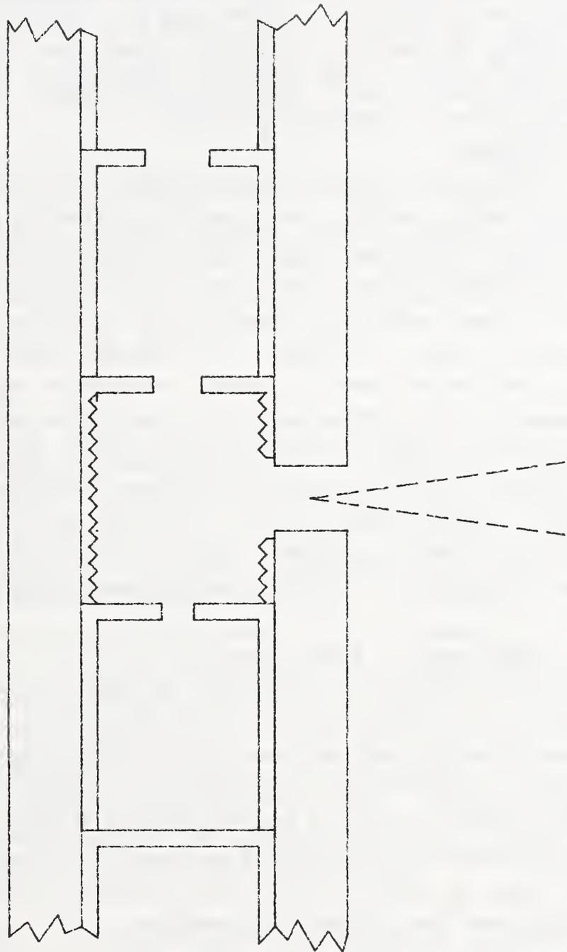
FIGURE 3. Central Section of Variable Temperature Blackbody
