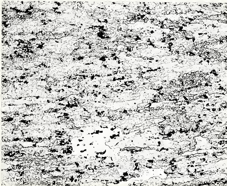
Figure 6. Longitudinal microstructure immediately adjacent to origin of fracture. Keller's etch. X 100
