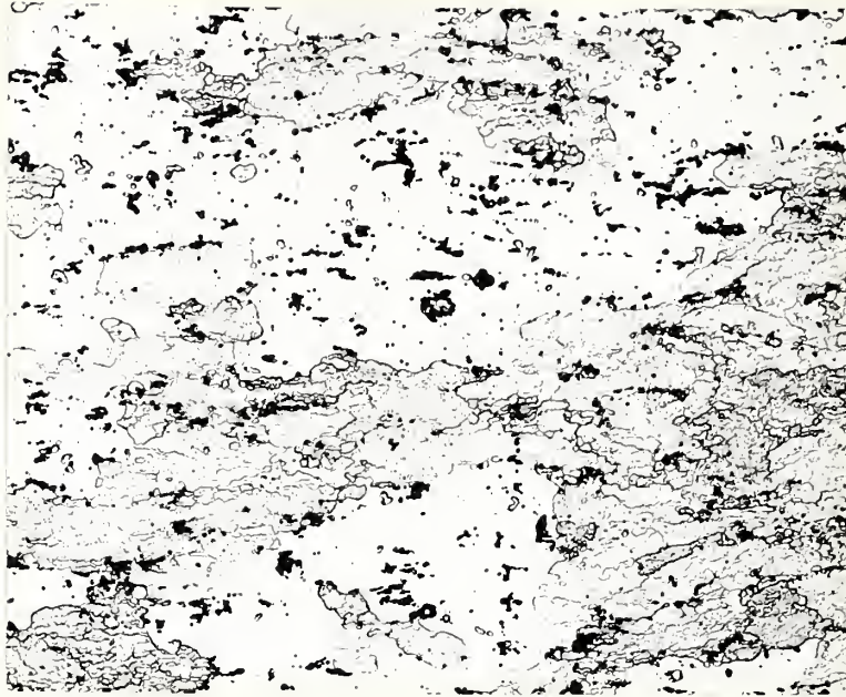
Figure 7. Microstructure of longitudinal section away from fracture. Keller's etch. X 100
