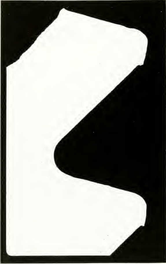
Figure 11a. Thread profile of hub socket No. 2 showing two damaged threads adjacent to fracture. X 18
