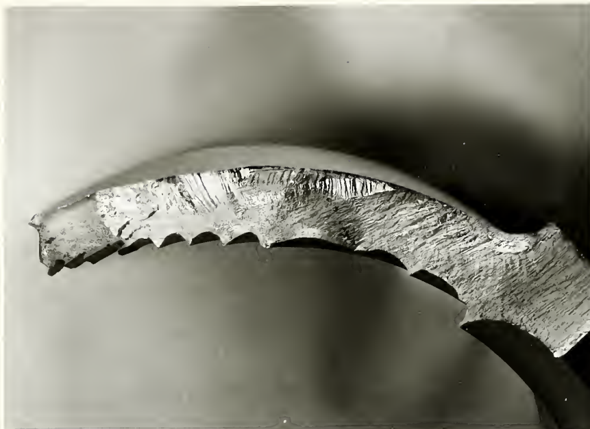
Figure 3. Fracture surface of failed hub socket, No. 2. X 1
