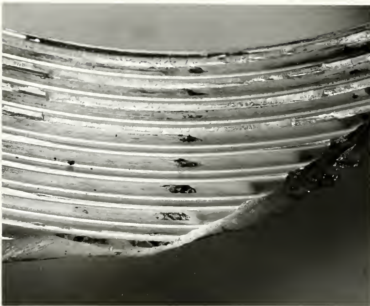
Figure 8. Threads of failed hub socket showing fretting. X 2
