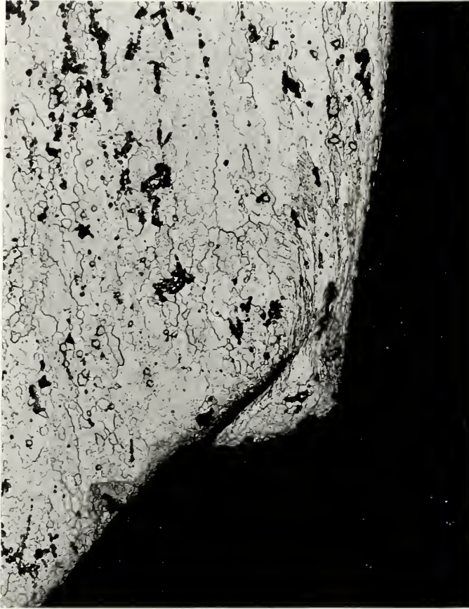
Figure 12. Thread adjacent to fracture in hub socket No. 2 showing deformation. Keller's etch. X 200
