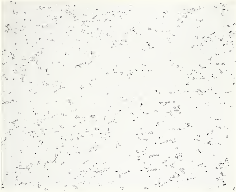
Figure 5. Representative longitudinal area adjacent to origin of fracture. Unetched. X 100
