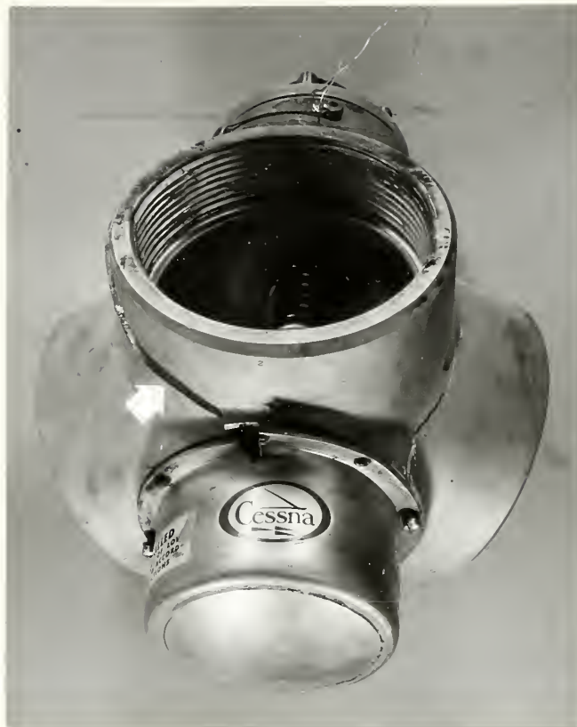
Figure 1. McCauley Propeller Hub as received. Arrow on photograph points to approximate location of fracture origin on inside of hub. X 3/8
