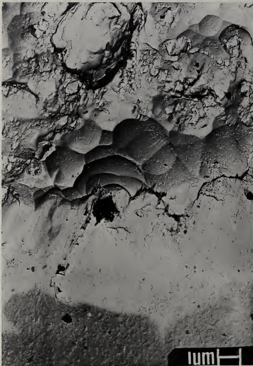
Fig. 2 6,900X. 6061 pickled with resulting good spall resistance. Keller's Etch was given in two 15 sec. exposures, each exposure followed by a very light buff on a felt polishing wheel.
