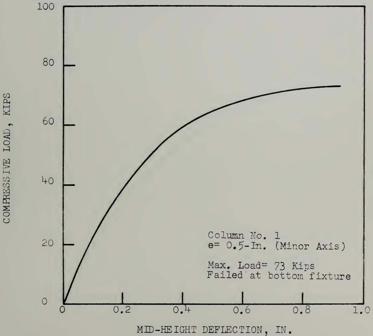
FIG. 10.3 SHORT-TERM TEST ON COLUMN NO. 1
