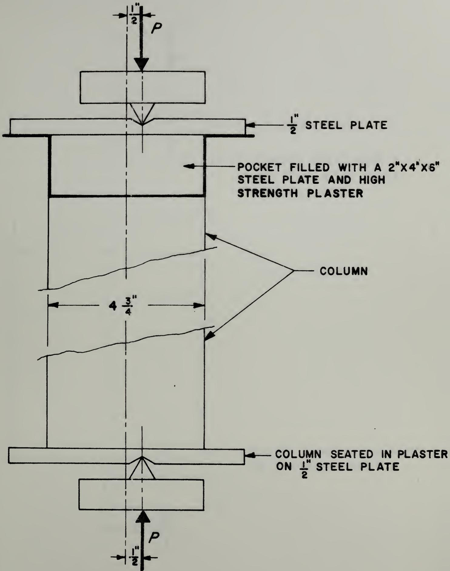
FIG. 10.1. TEST METHOD FOR COLUMN TESTS (Minor Axis)
