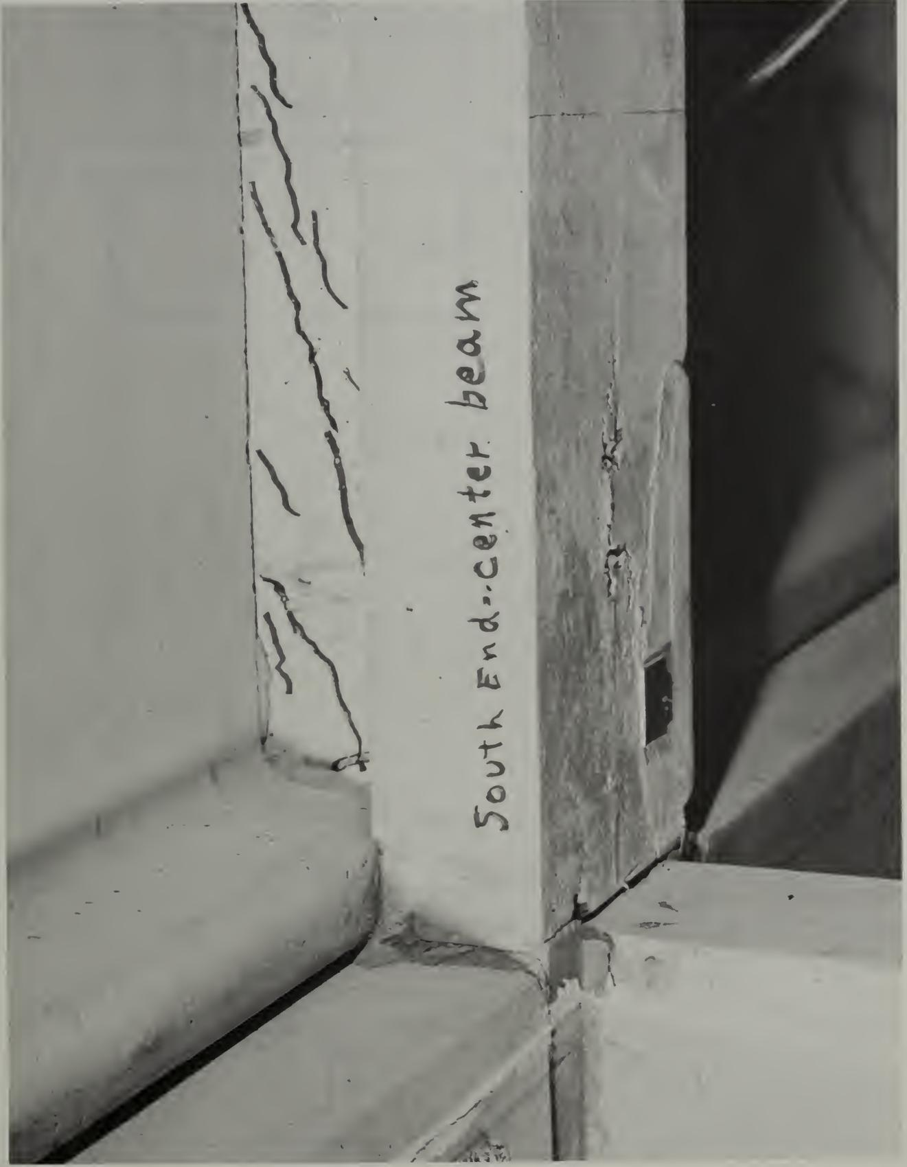
Fig. 9.23 Diagonal tension cracking at  $W=270$  PST
