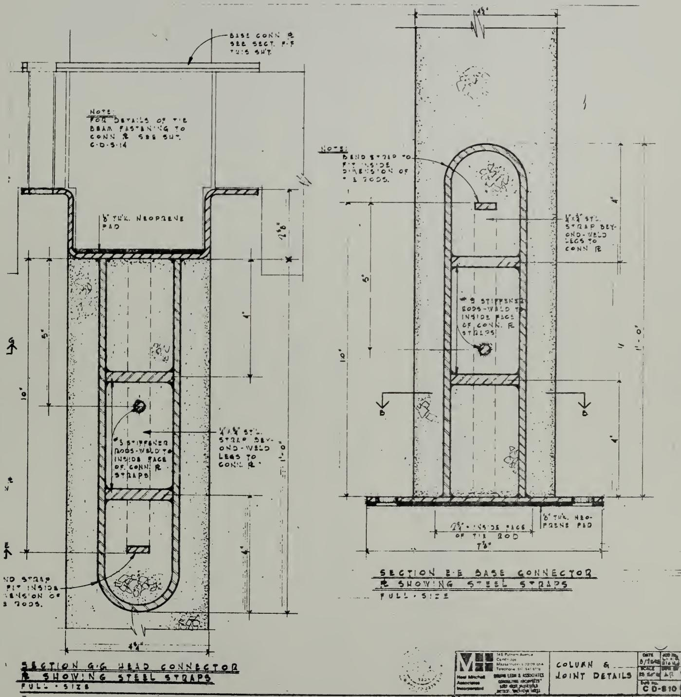
Fig. 5.5 Column head and base plate connectors
