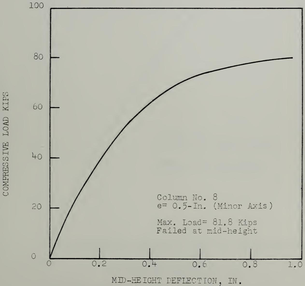
FIG. 10.5 SHORT-TERM TEST ON COLUMN NO. 8
