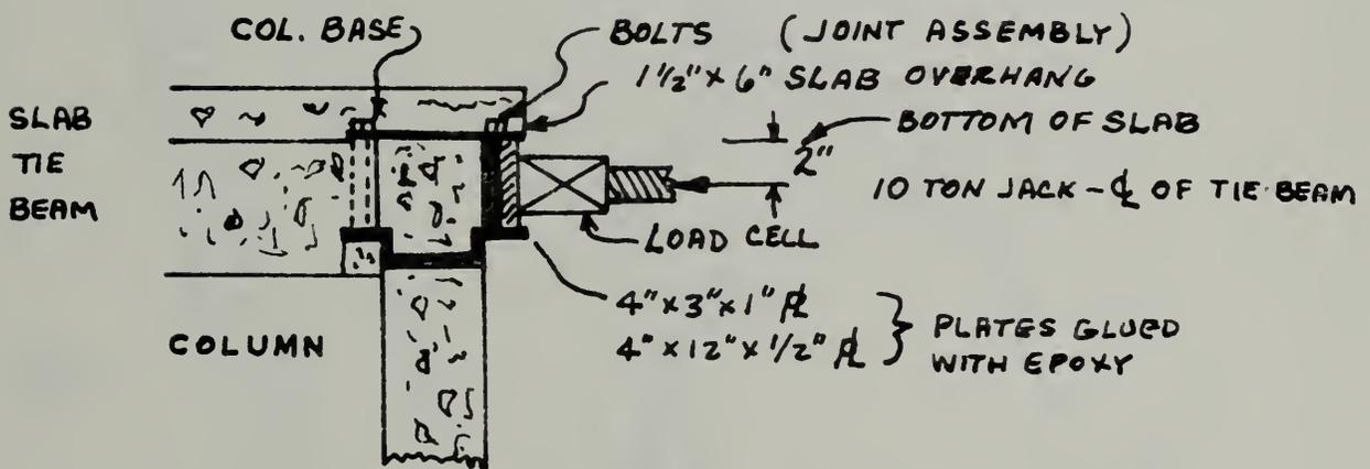
FIGURE 6.4 TYP. W → E RACKING LOAD
