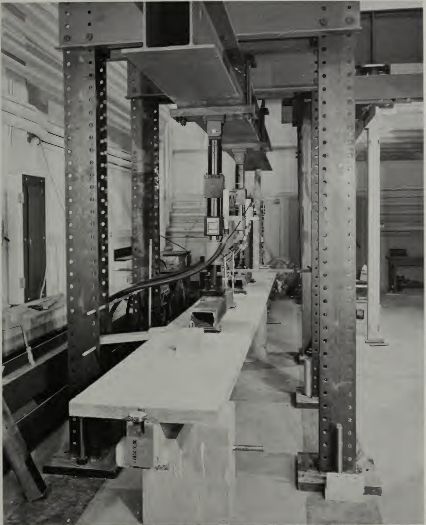
Fig. 10.14 Fatigue test on main beam
