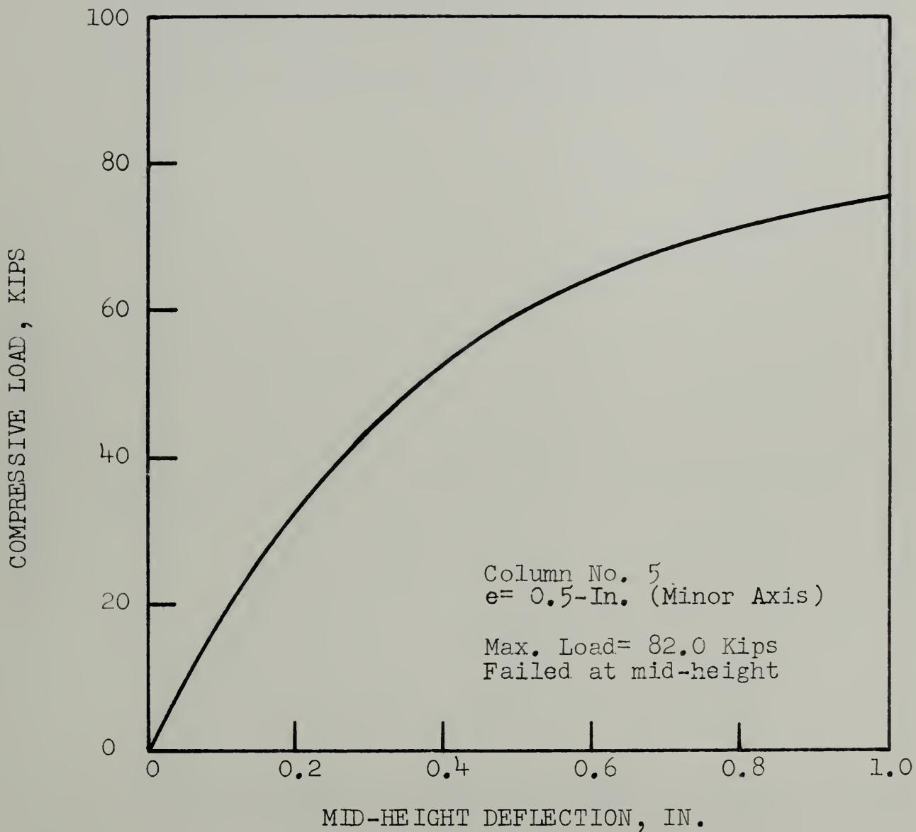
FIG. 10.4 SHORT-TERM TEST ON COLUMN NO. 5
