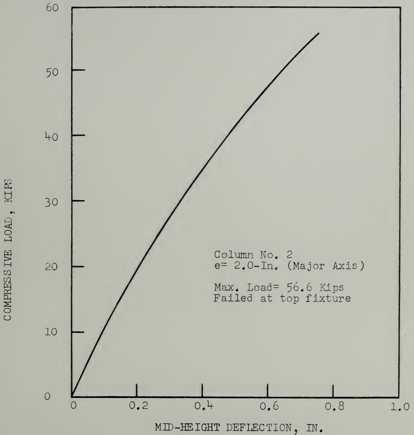
FIG. 10.6 SHORT-TERM TEST ON COLUMN NO. 2
