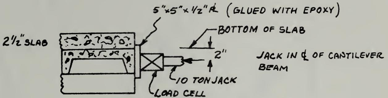
FIGURE 6.3 TYP. N → S RACKING LOAD
