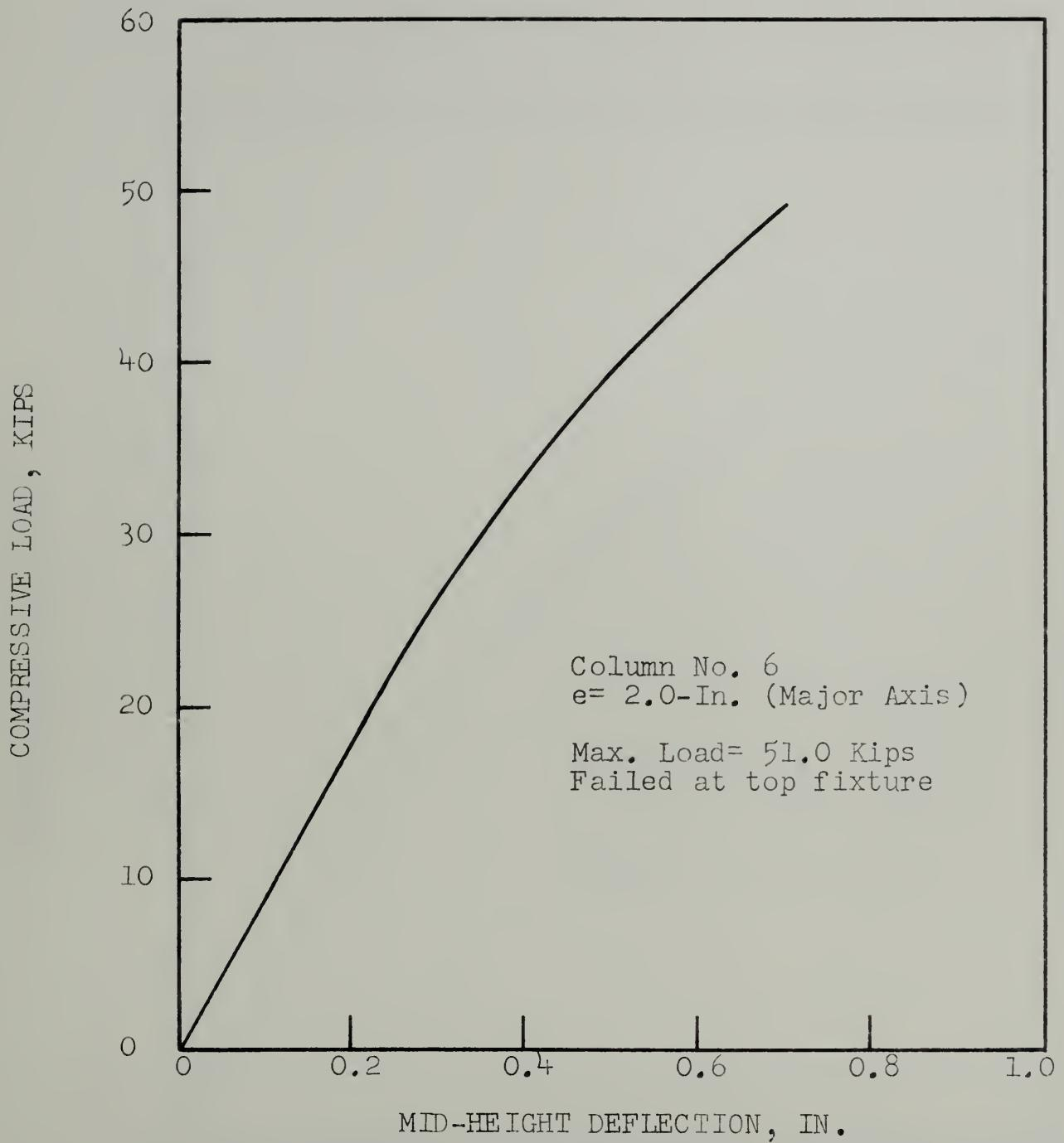
FIG. 10.7 SHORT-TERM TEST ON COLUMN NO. 6
