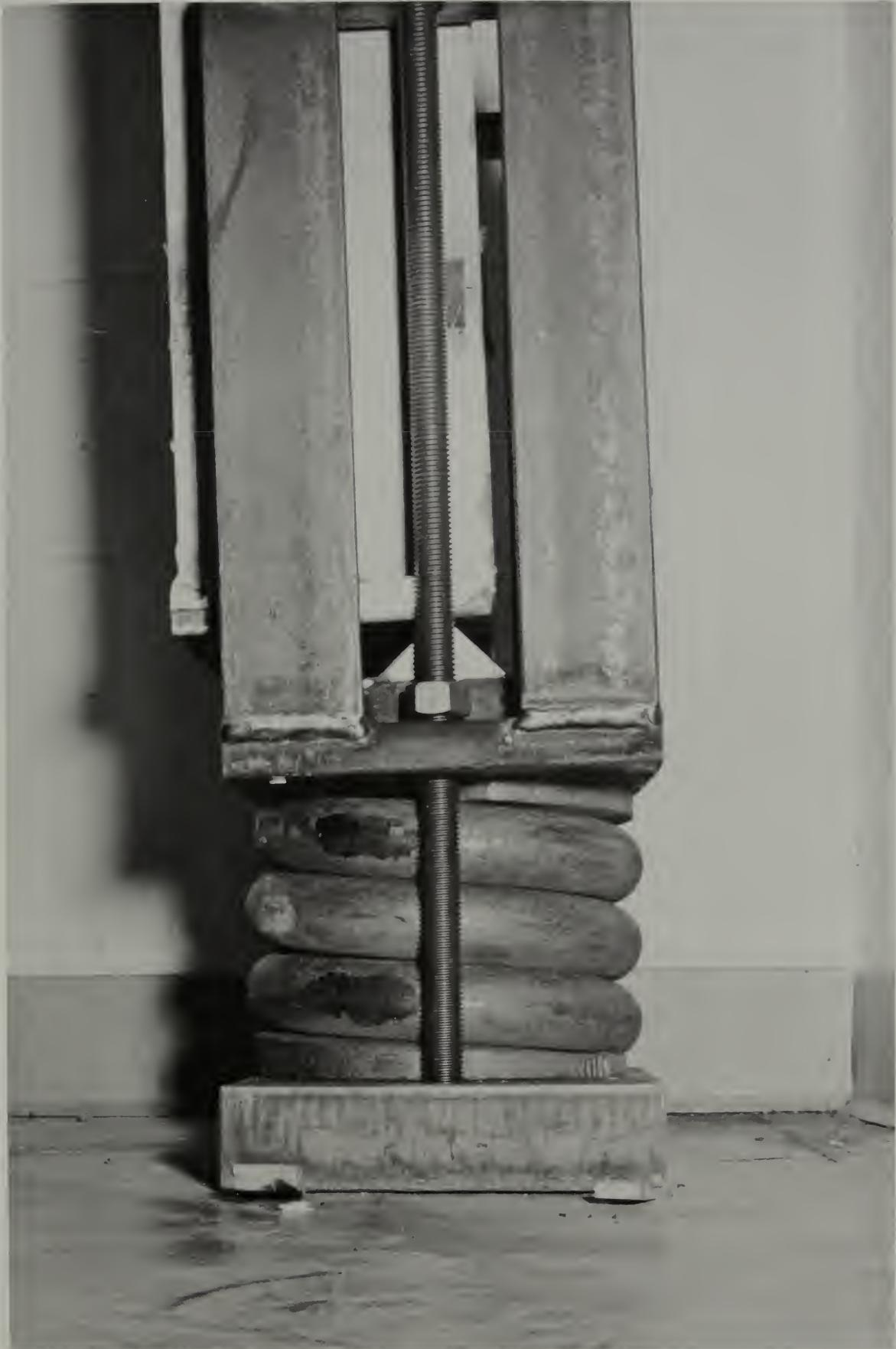
Fig. 10.11 Detail of base for column No. 4 creep frame
