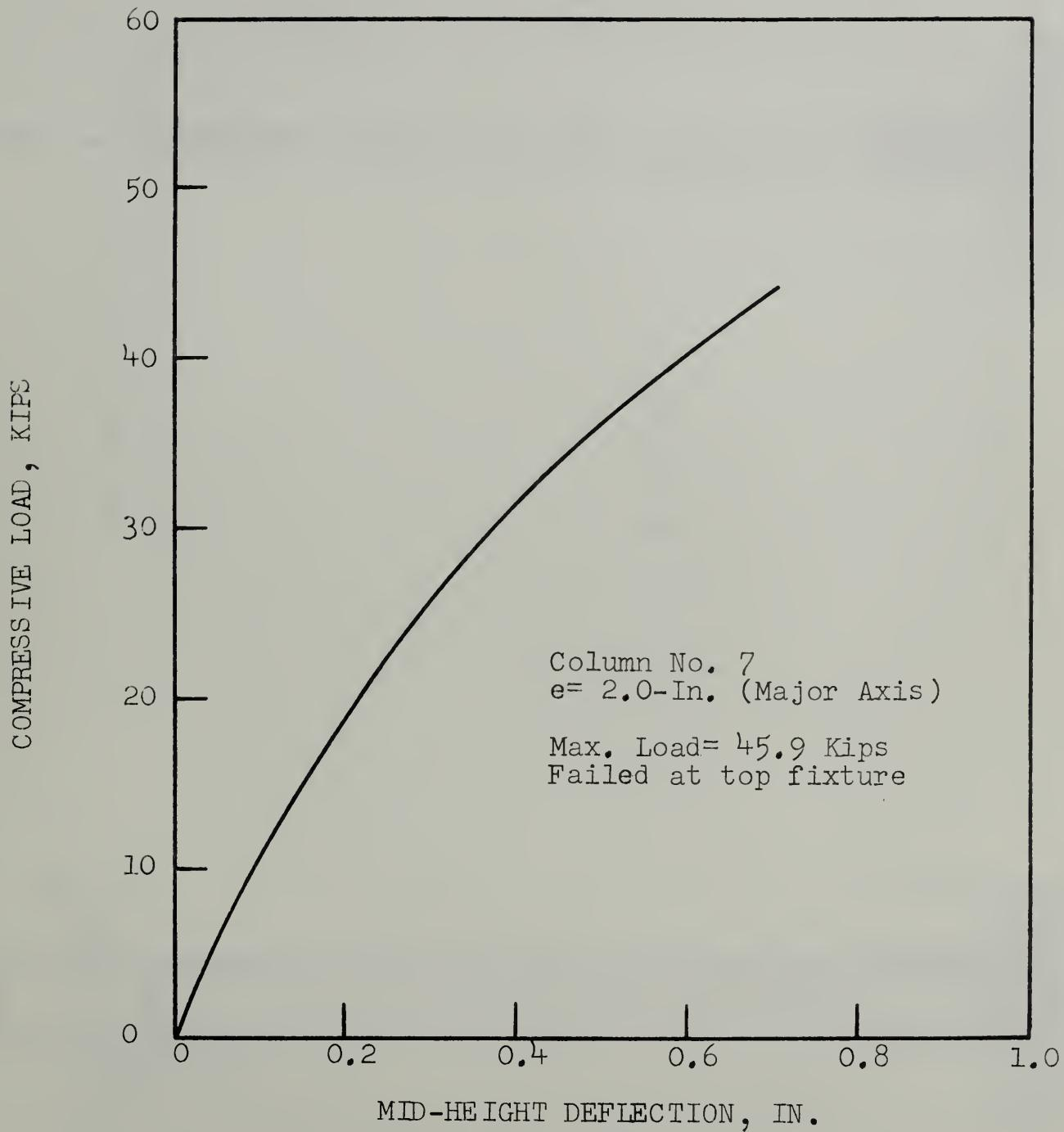
FIG. 10.8 SHORT-TERM TEST ON COLUMN NO. 7
