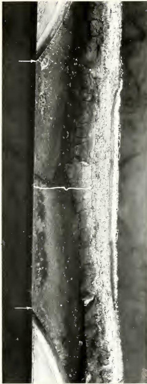
Figure 3. Fracture surface of failed printing plate. Arrows point to apparent crack origins. The surface is typical of that resulting from fatigue. The depth to which the crack propagated is bracketed. X 8
