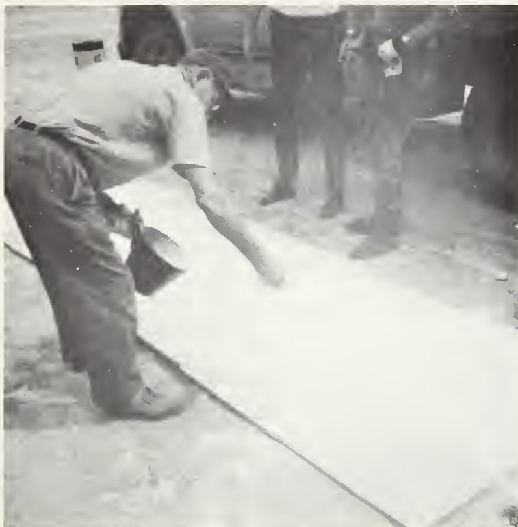
FIGURE 1. Coating of insulation boards with lime dust to prevent adhering of field samples.
