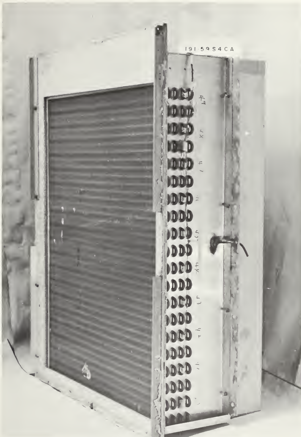
Figure 17. Air inlet and left end of Size IV evaporator (NBS No. 191-59) as mounted for test.
