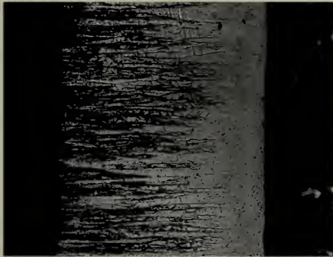
Figure 3. Microstructures in transverse sections of electrodeposited nickel-iron plates. Nickel deposit is shown. Principal grain axes are normal to plate surfaces. Note unetched iron-rich layer adjacent to nickel-iron interface. Etched with Carapella's reagent. X 250.
