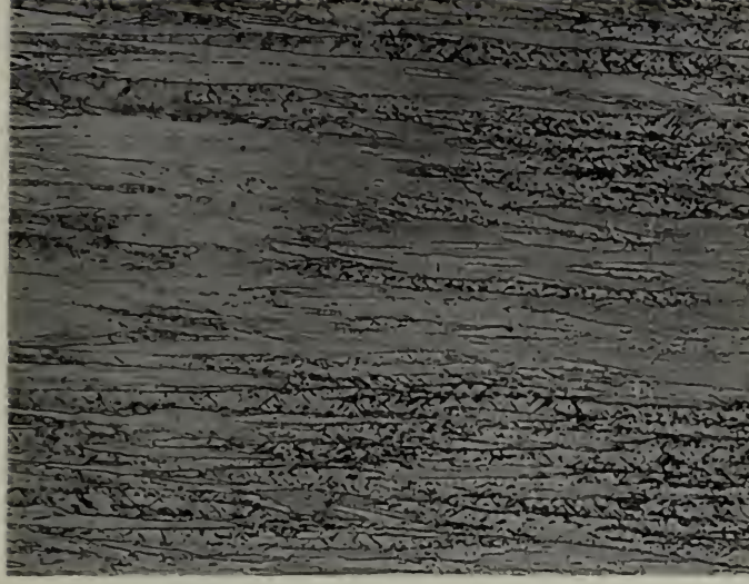
Figure 2. Microstructures in transverse sections of electroformed nickel plates. Principal grain axes are normal to plate surfaces. Etched with Carapella's reagent. X 250.
