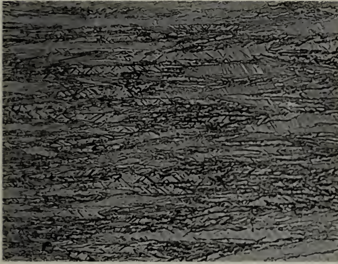
Figure 2. Microstructures in transverse sections of electroformed nickel plates. Principal grain axes are normal to plate surfaces. Etched with Carapella's reagent. X 250.
