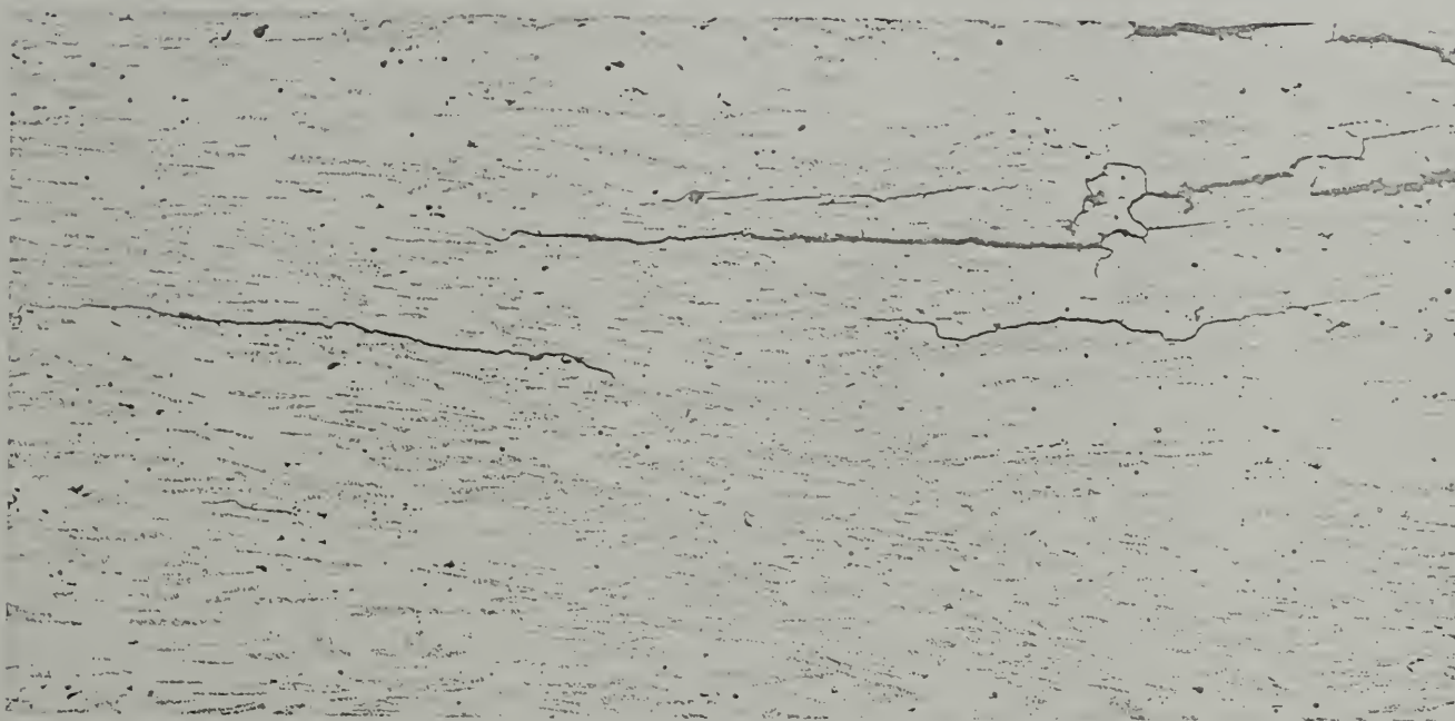
Figure 1. Secondary cracks observed on failed "C" ring specimen stressed at 75% of the alloy yield strength. Note that cracks are intergranular and braching in nature.
