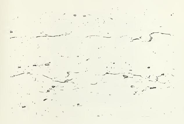
Photomicrograph of a 2219-T87 aluminum alloy short transverse tensile specimen prior to testing. Photomicrograph was taken at the same level as indicated by fractures in Figure 1. Unetched X 100
