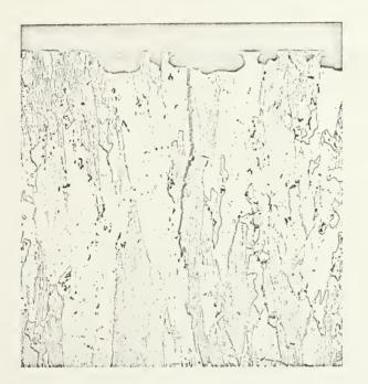
Photomicrograph of a 7075-T651 aluminum alloy short transverse specimen which failed at 75% of its yield strength after 5 minutes in Alcoa H solution. Note the intergranular stress-corrosion cracks which start at the pits. Keller's etch X 100
