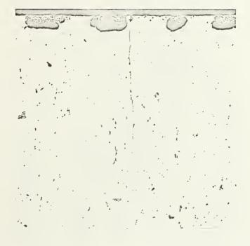
Photomicrograph of a 7075-T651 aluminum alloy short transverse specimen which failed at 75% of its yield strength after 5 minutes in Alcoa H solution. Unetched X 100
