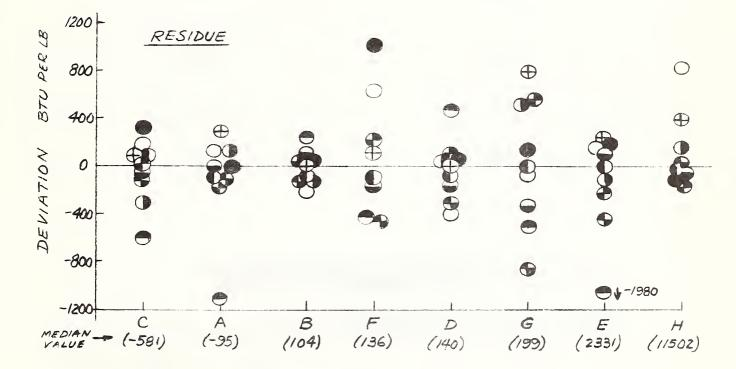
FIGI. <u>DEVIATION FROM MEDIAN HEAT OF COMBUSTION</u> VALUE FOR EACH MATERIAL
