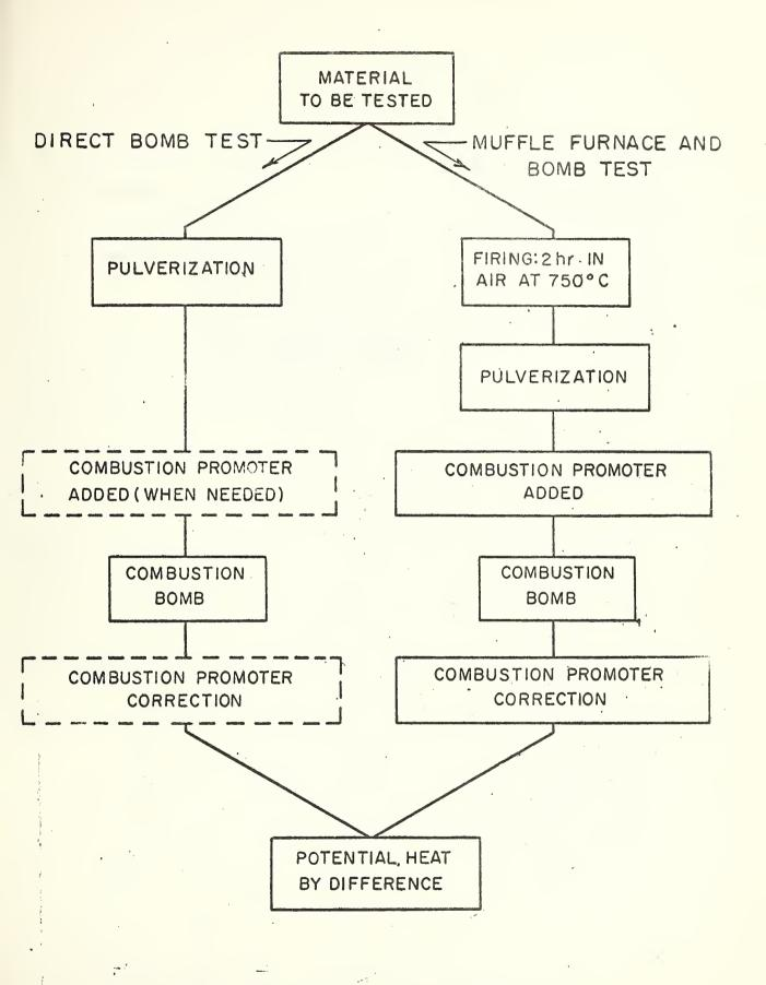
Figure 1A. Schematic Diagram of Test Procedure for Potential Heat Measurements
