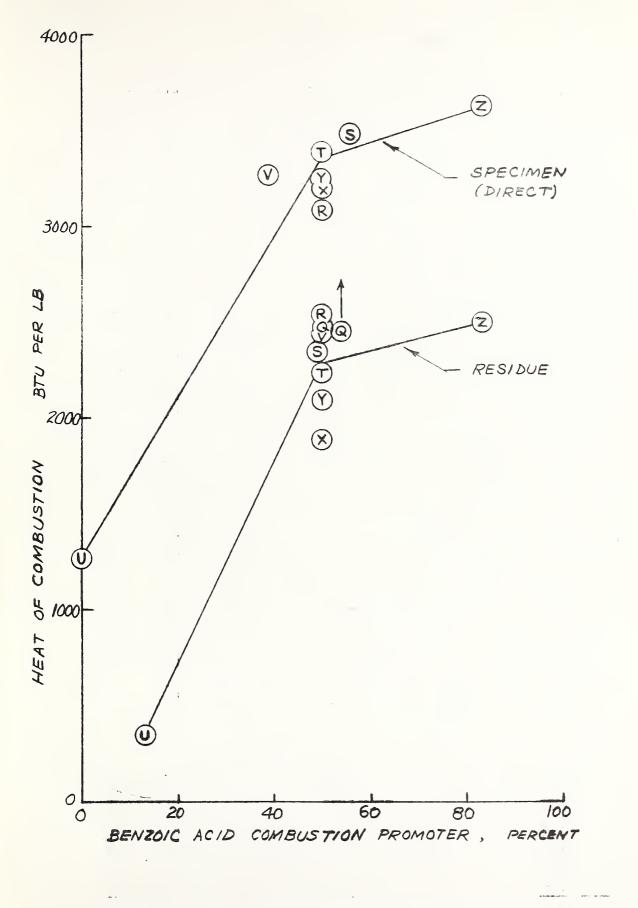
FIG.3 SPECIMEN AND RESIDUE HEATS OF COMBUSTION FOR MATERIAL E
