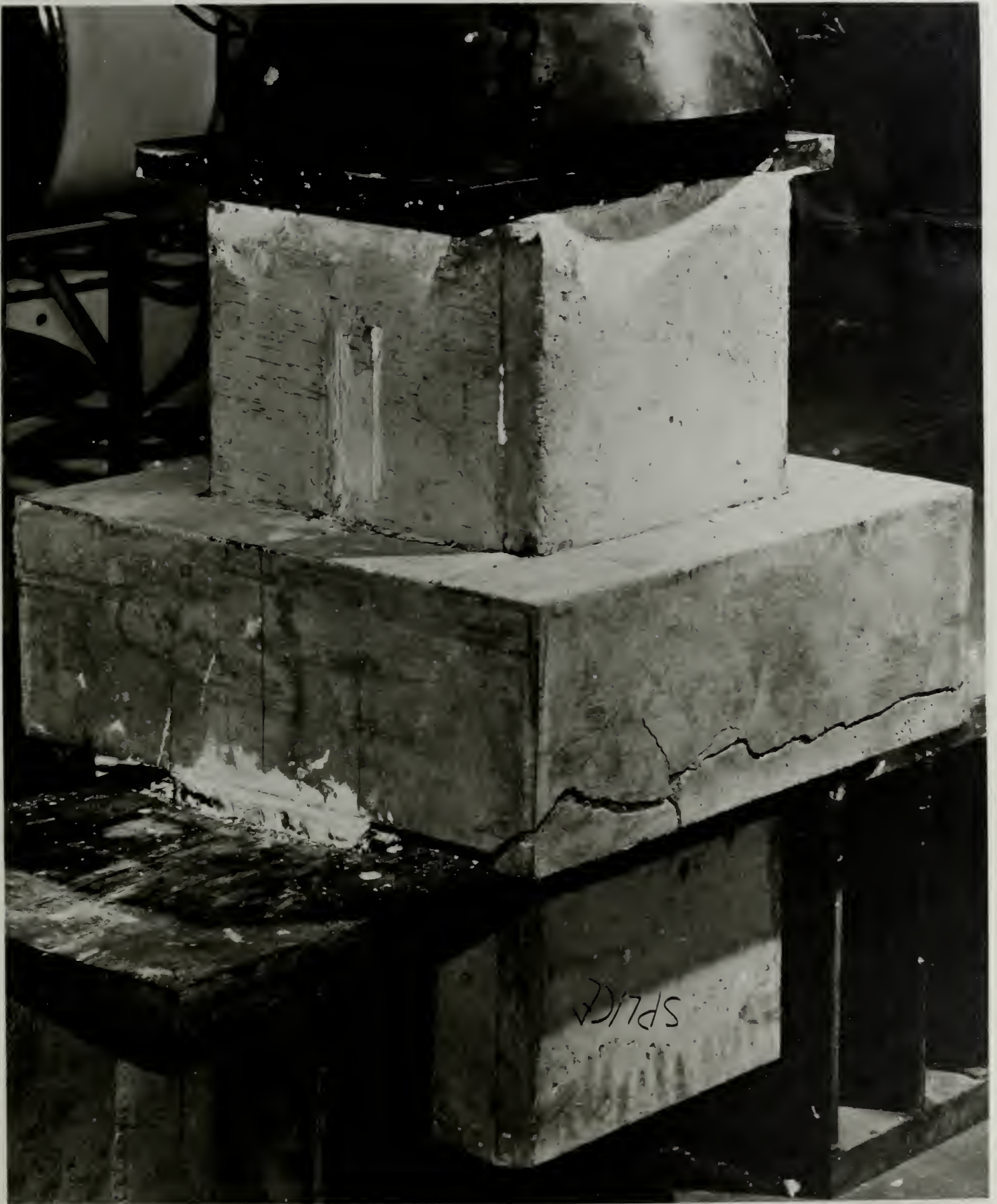
FIG. 4. COLLAR No. 2 AT FAILURE.
