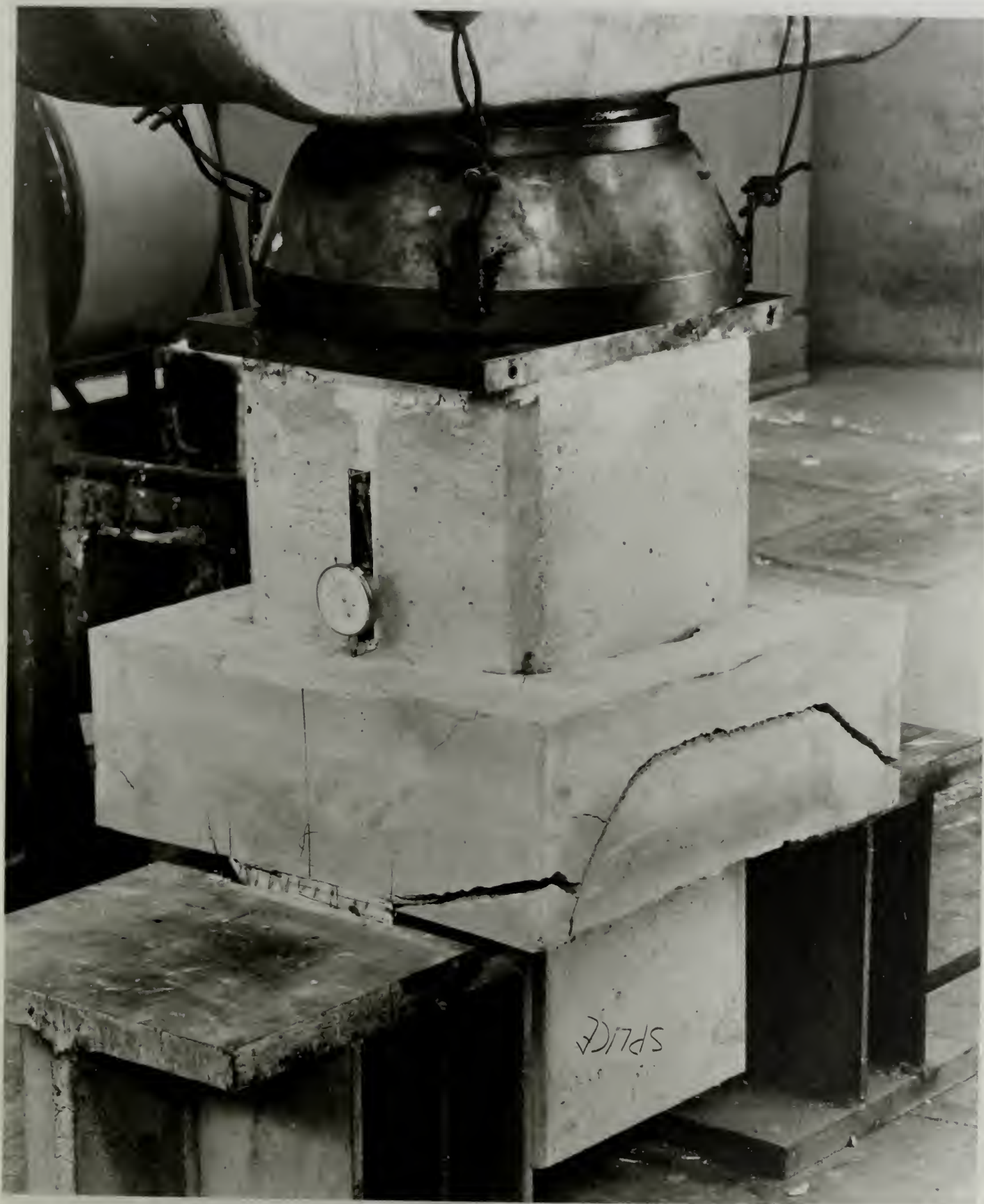
FIG. 3. COLLAR No. 1 AT FAILURE.
