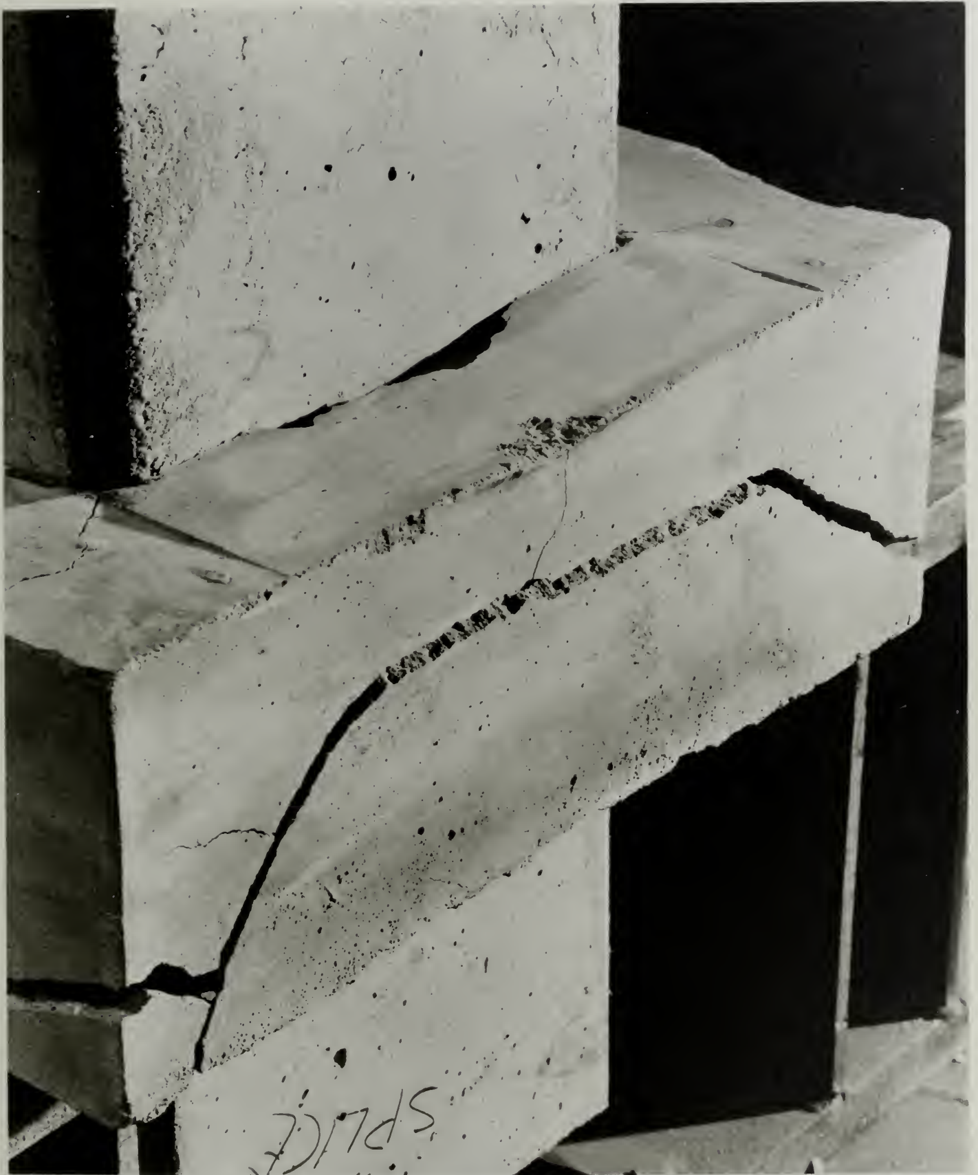
FIG. 2. CLOSE-UP OF COLLAR No.1 AFTER FAILURE.
