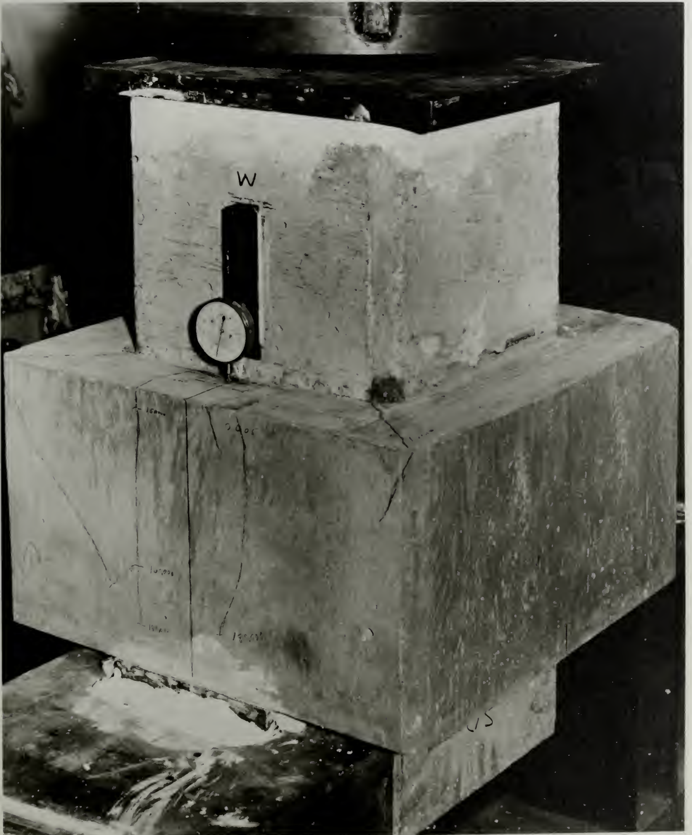
FIG. 5. COLLAR No. 3 AT FAILURE.
