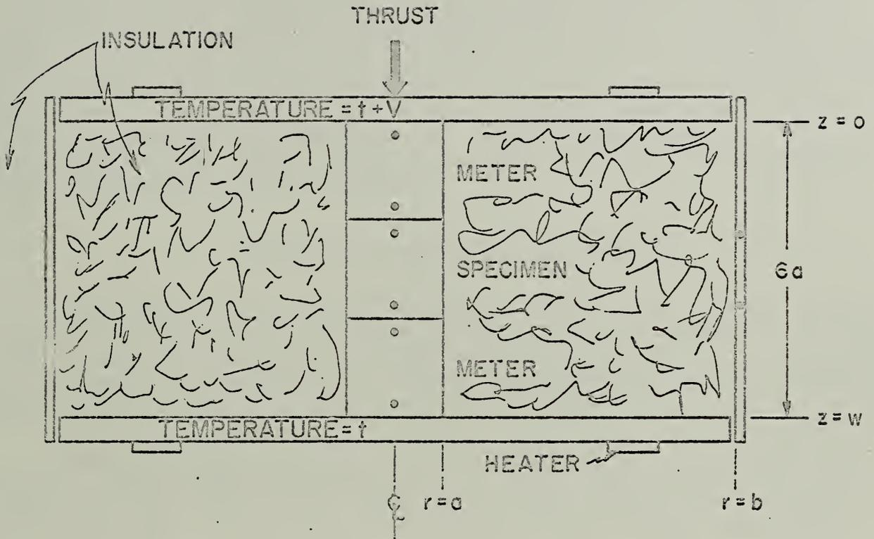
FIGURE 4. SCHEMATIC FOR A GUARDED CUT-BAR APPARATUS DESIGNED FOR CALIBRATION OF METERS BY MEANS OF THERMAL CONDUCTIVITY REFERENCE SPECIMENS, WITH THE CALIBRATION SUBSTANTIALLY INDEPENDENT OF PRECISE GUARD TEMPERATURE MANAGEMENT
