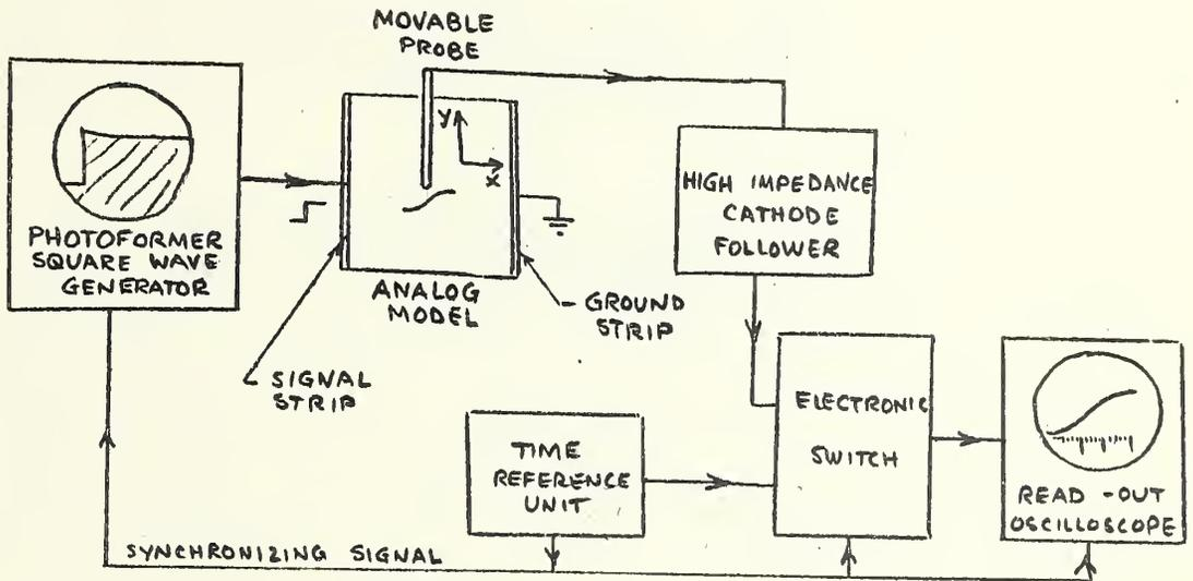
Figure 1. Schematic diagram for measurement of the time constant of a continuous-resistance, continuous-capacitance analog.
