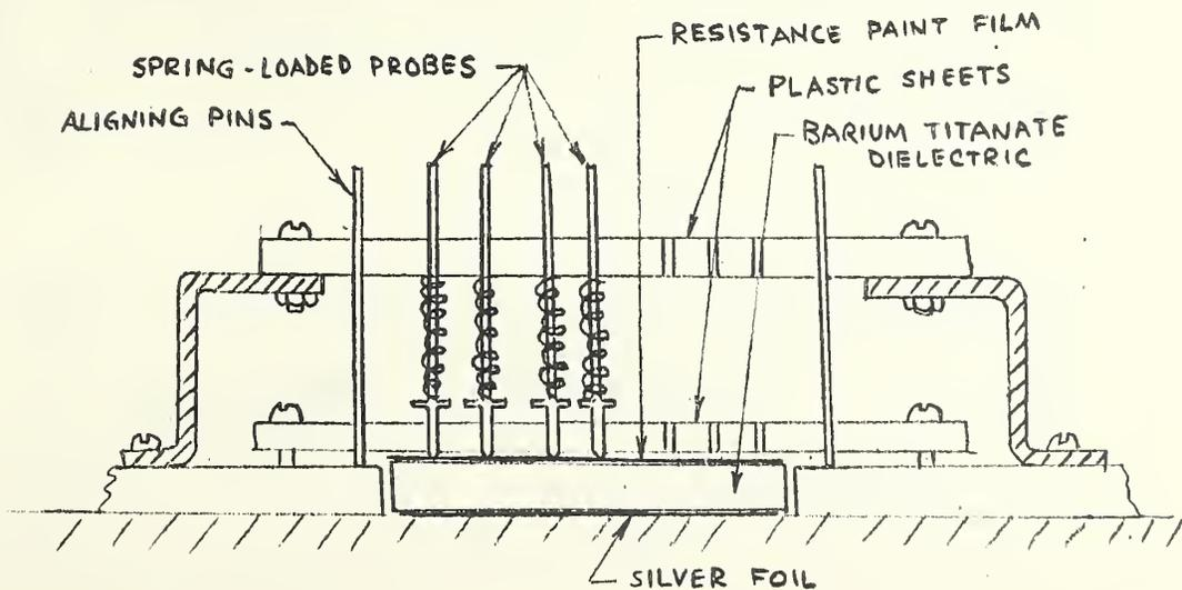
Figure 2. Mounting details of analog model
