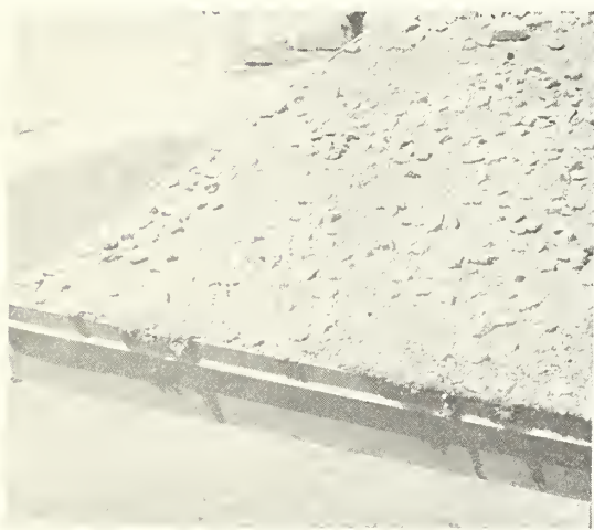
FIGURE 8. FLOW OF SURFACING ASPHALT.
