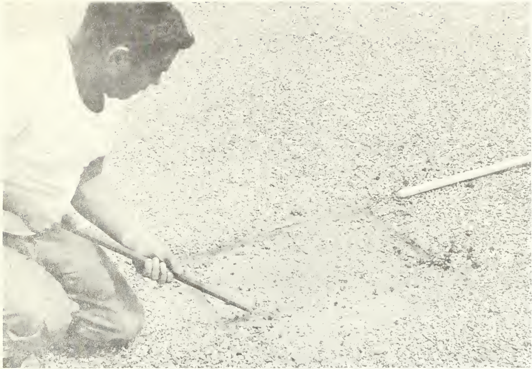
FIGURE 2. REMOVAL OF A CUT-OUT SPECIMEN.
