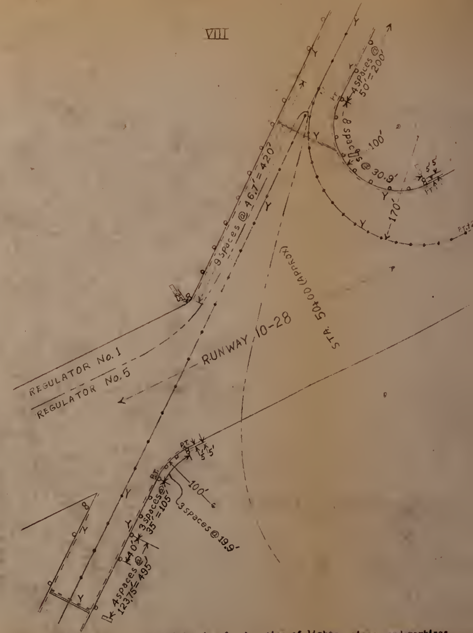
Figure 2-VIII. Detailed drawing for location of lights, signs, and markings for taxiways in area VIII.
