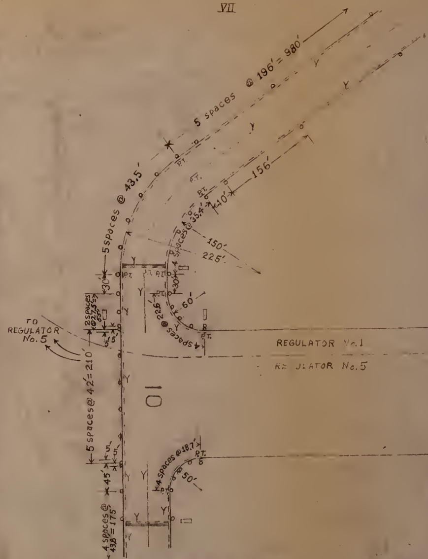
Figure 2-VII. Detailed drawing for location of lights, signs, and markings for taxiways in area VII.
