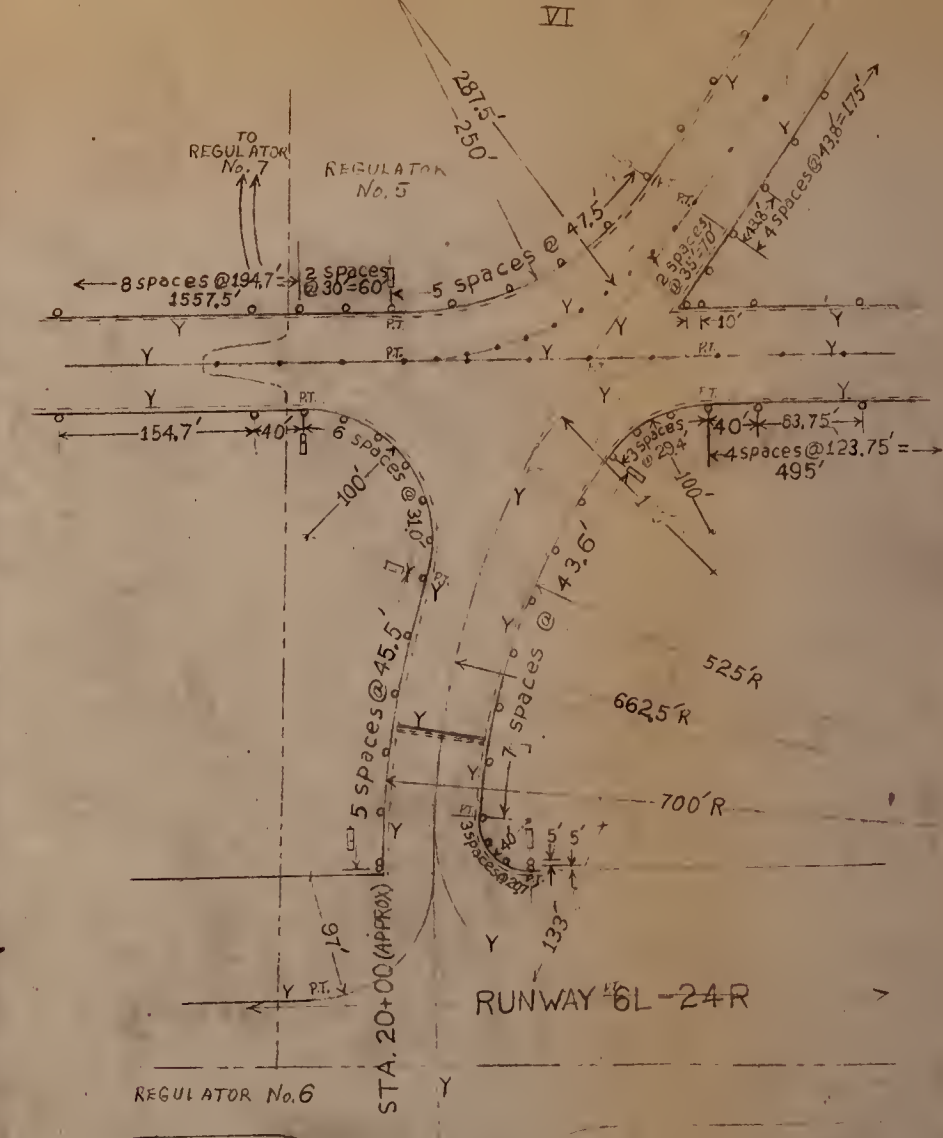
Figure 2-VI. Detailed drawing for location of lights, signs, and markings for taxiways in area VI.
