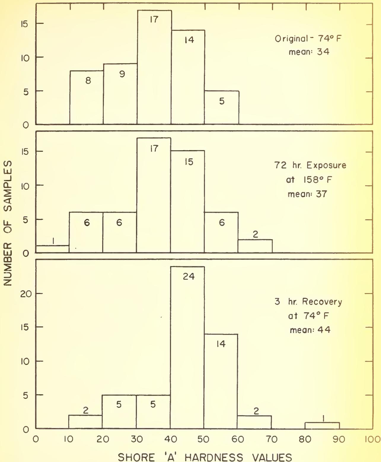
FIG. 6 DISTRIBUTION OF SHORE 'A' HARDNESS VALUES OBTAINED ON 53 SPECIMENS OF RUBBER BASE CALKINGS.
