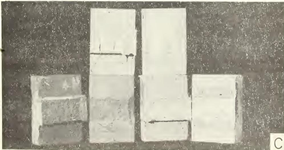
Fig. 14. Bond-ductility test specimens. (A) Typical specimens before test: brick, concrete block, concrete and wood. (B) Examples of complete bond failure after test. (C) Failure caused by combination of high hardness of calking and strong adhesion resulting in breakage of the accessory blocks
