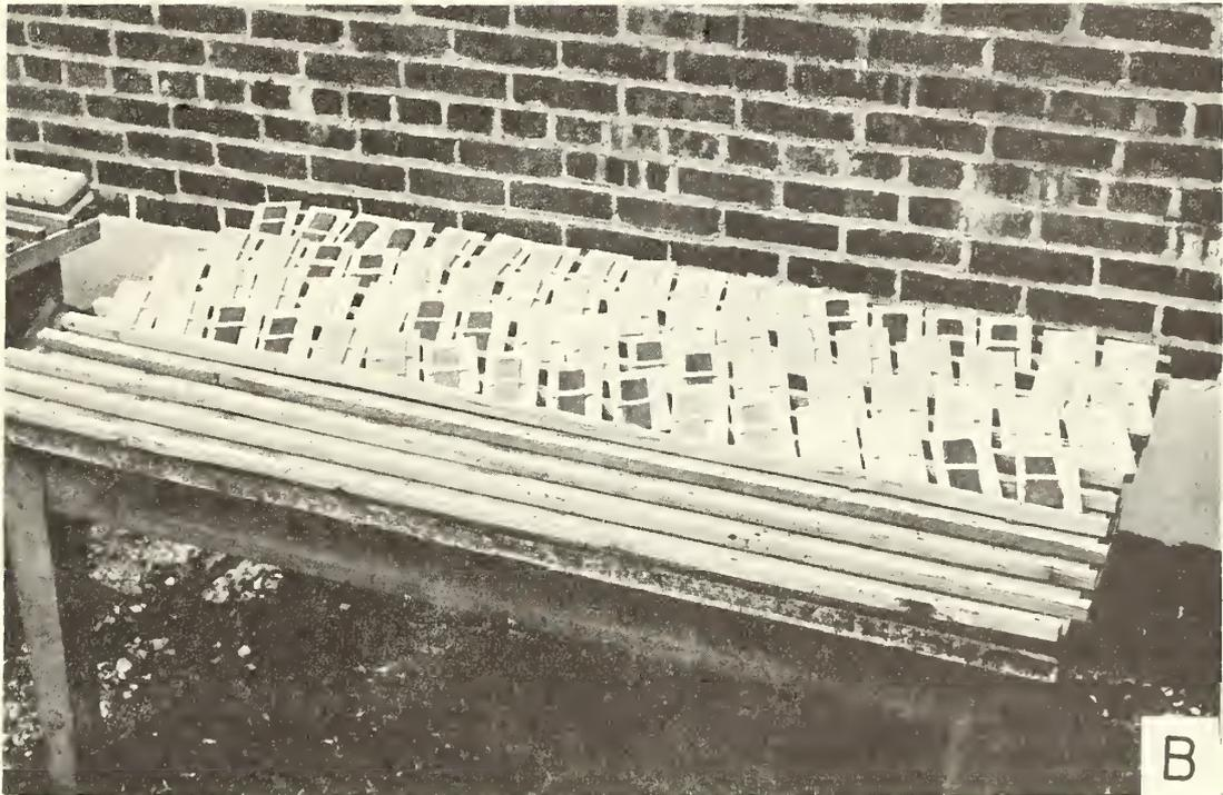
Fig. 4. Calking specimens used for the determination of Shore A hardness.
