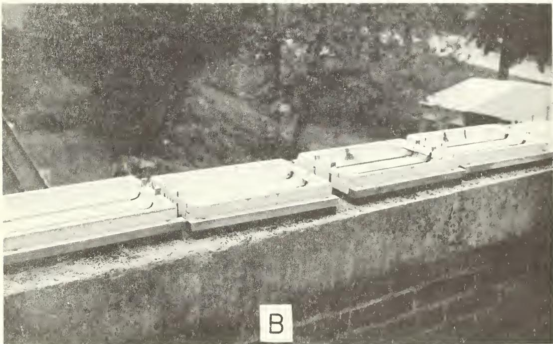
Fig. 15. Calked joints used in outdoor exposure studies.
