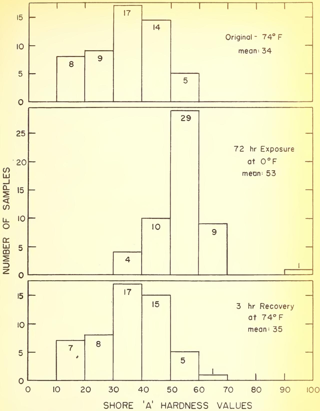
FIG. 5 DISTRIBUTION OF SHORE 'A' HARDNESS VALUES OBTAINED ON 53 SPECIMENS OF RUBBER BASE CALKINGS.
