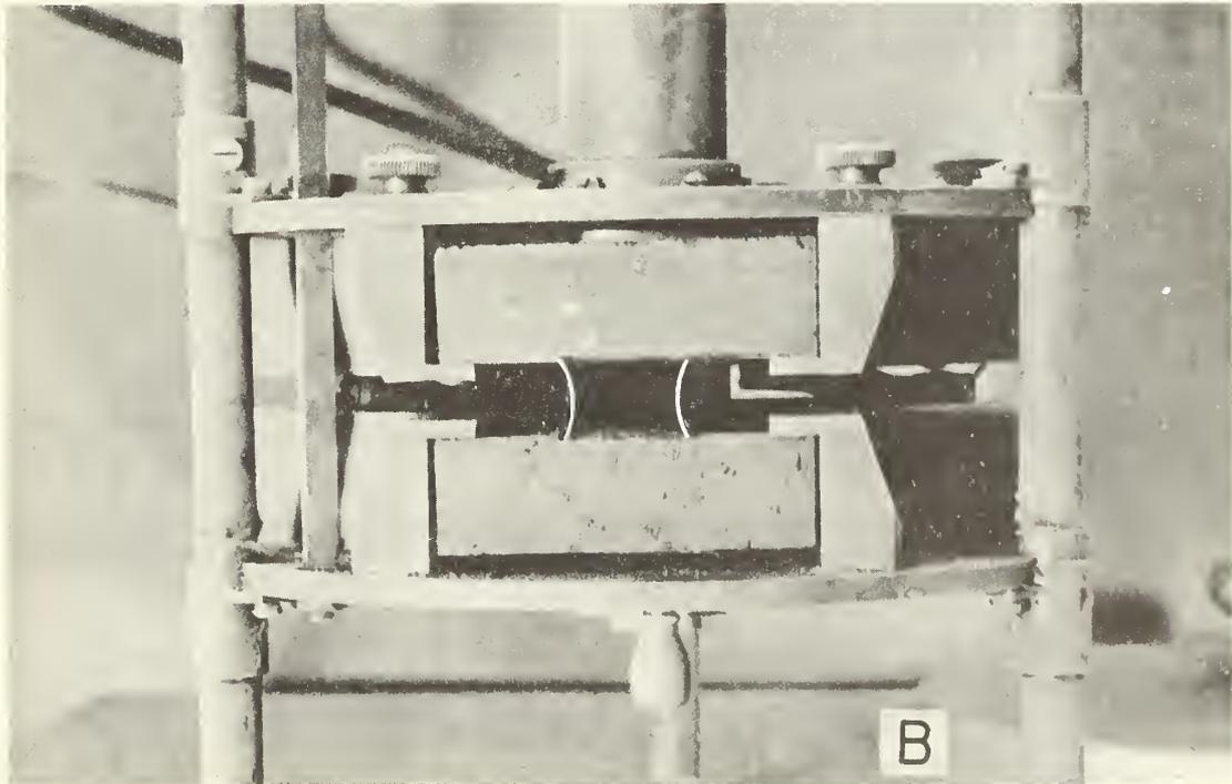
Fig. 13. Bond-ductility test specimens in joint material extension machine.
