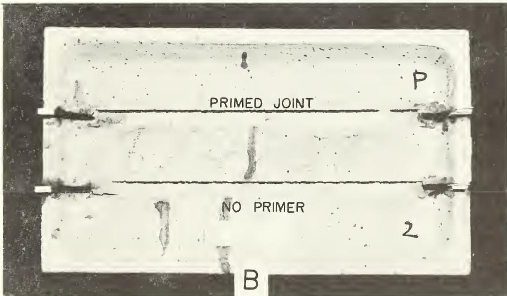
Fig. 16. Effect of six months exposure to the weather on calkings in concrete joints. Joints were stretched total of  $3/32$  in.
