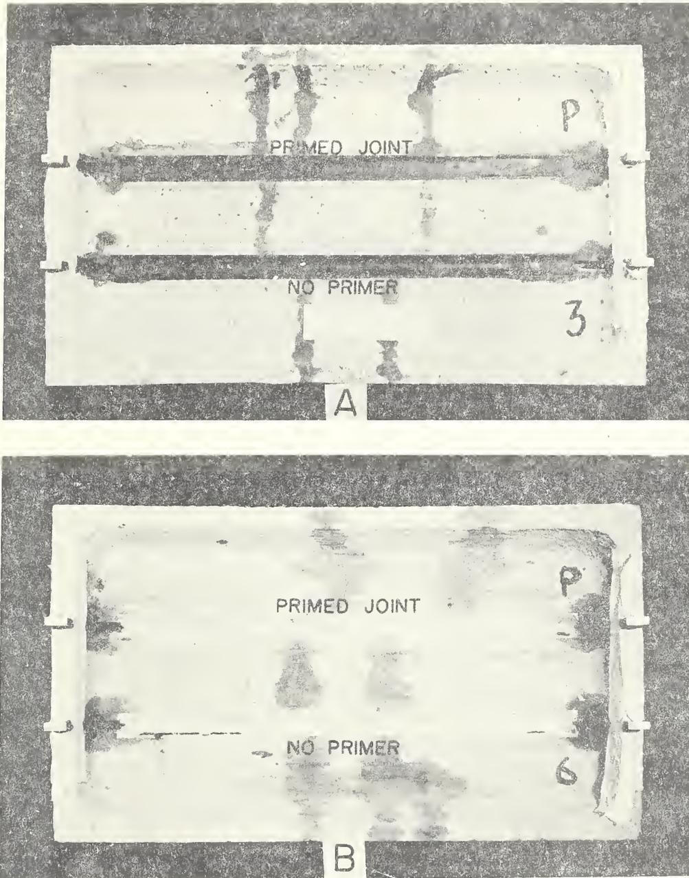
Fig. 17. Effect of six months exposure to the weather on two samples of calkings in concrete joints. Joints were stretched a total of  $\frac{3}{32}$  in.
