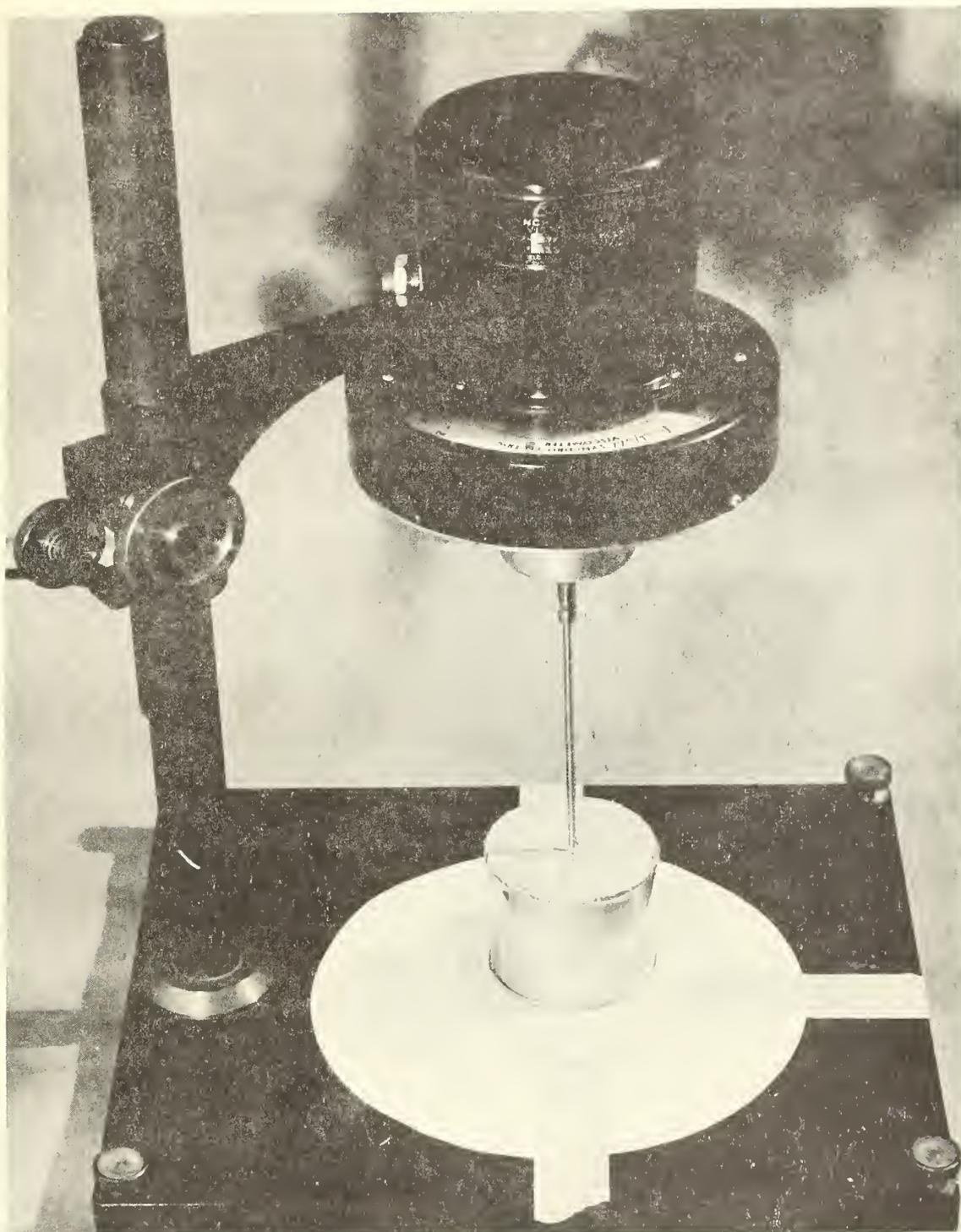
Fig. 7. Application or "pot" life of the calkings was measured with a Brookfield Viscometer fitted with no. 7 spindle rotating at 2 rpm. Readings were taken periodically and test was stopped when pointer reached the limit of the scale (100) or after 180 minutes- whichever came first.
