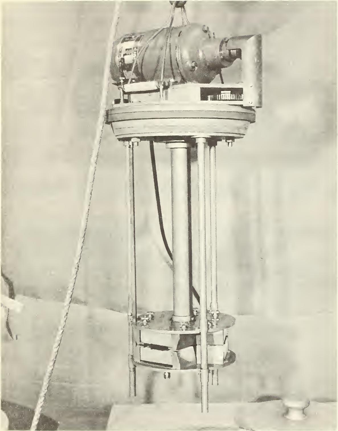
Fig. 12. Joint material extension machine used in the bond-ductility tests. Joint is stretched 50% of its original width at 0 deg F, at the rate of  $1/8$  in. per hour.
