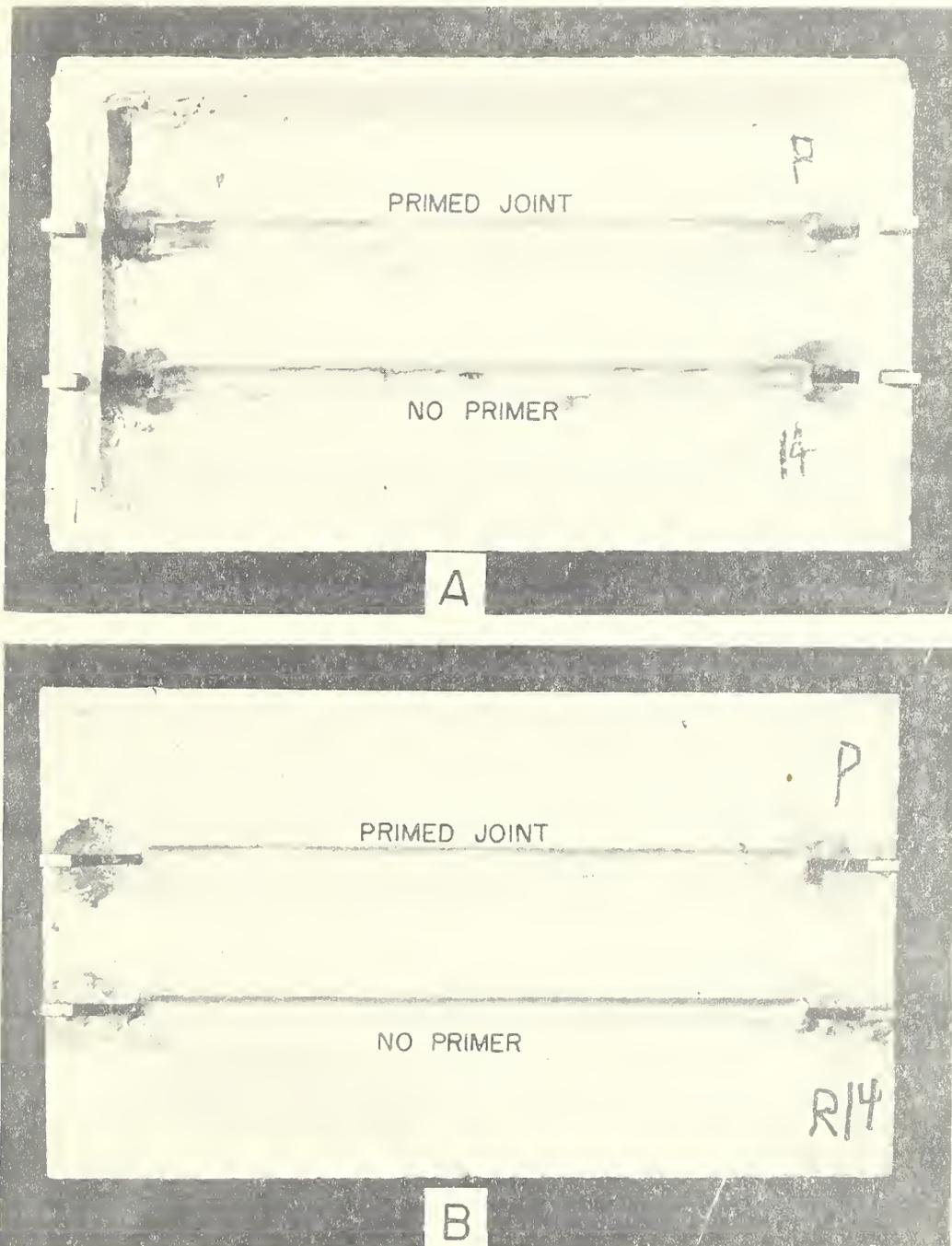
Fig. 20. Effect of six months exposure to the weather on calking sample No. 8-B. Joints were stretched a total of  $3/32$  in.
