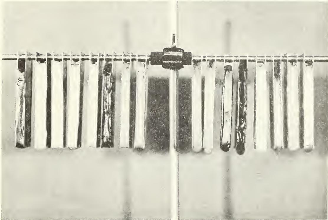
Fig. 3. Laboratory test of slump or flow property of rubber base calkings. Freshly mixed compounds are placed in aluminum troughs, 4 in. by 1 in. by  $\frac{3}{8}$  in. and are suspended for 24 hrs at ~~74<sup>o</sup> ± 2<sup>o</sup> for 24 hrs.~~  $122 \pm 2^{\circ}$  F. The eight specimens on the right side show varying degrees of slump while those on the left show none.
