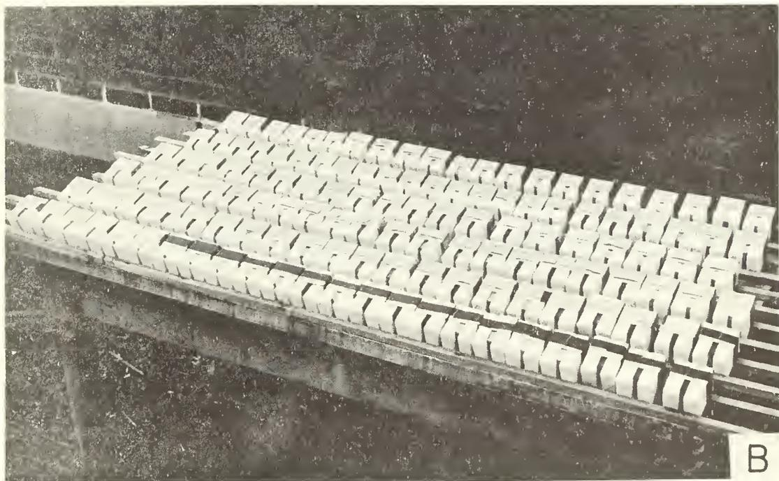
Fig. 2. Test specimens of rubber base calkings fabricated like those in Fig. 1, for study of staining of masonry and color changes in the calkings.
