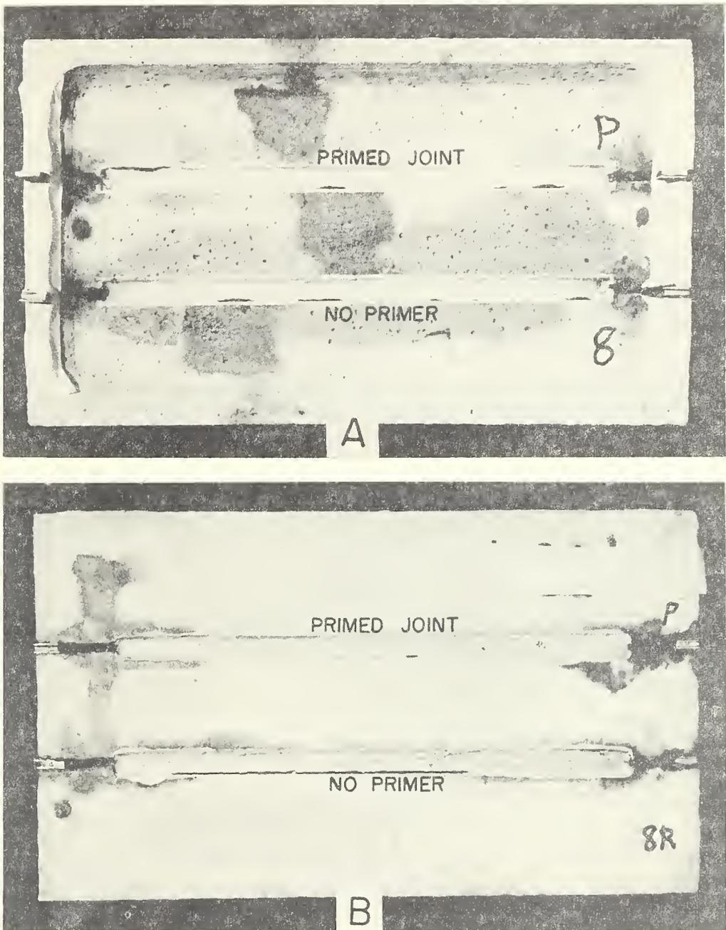
Fig. 18. Effect of six months exposure to the weather on a sample of calking in concrete joints (No. 15-B)
