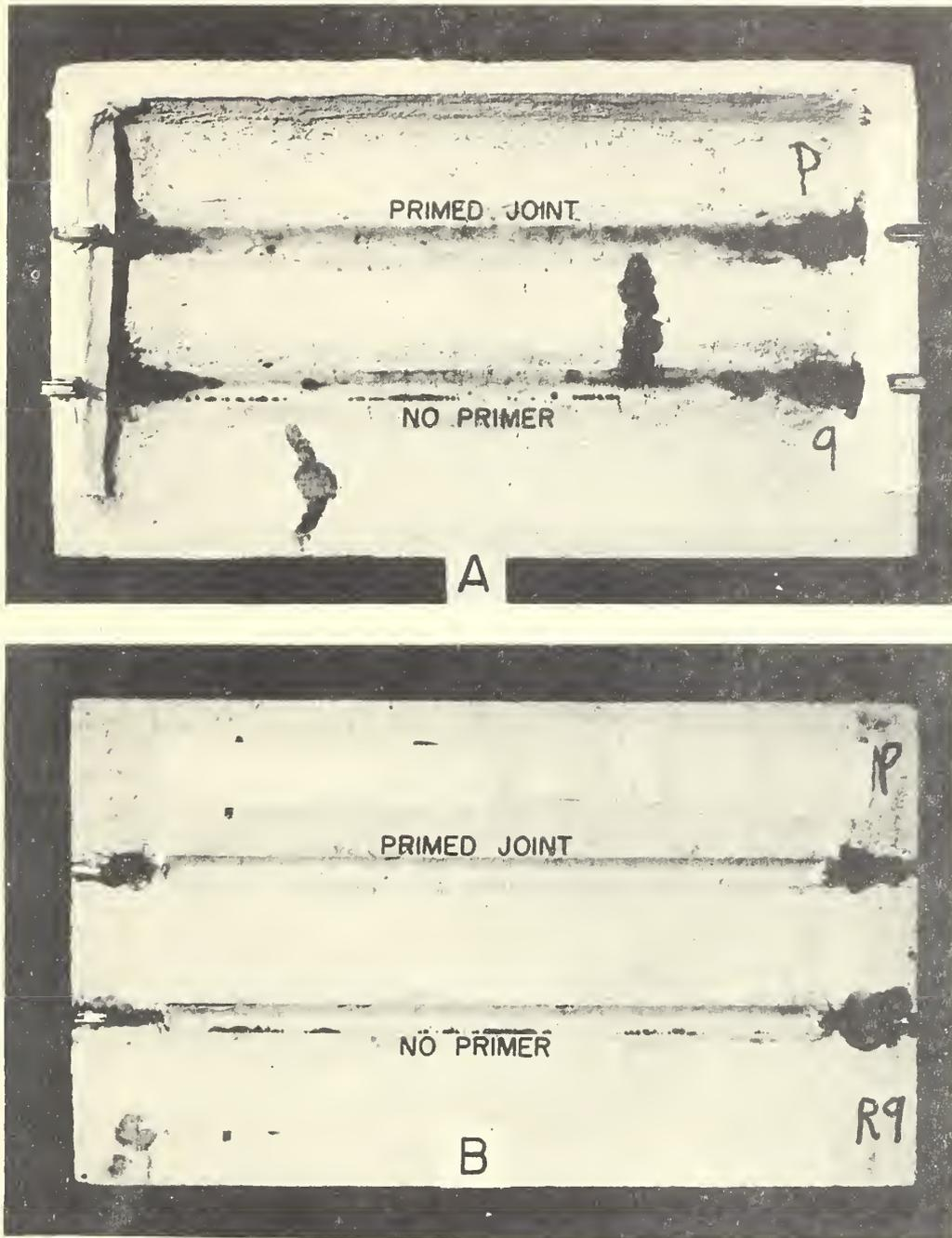
Fig. 19. Effect of six months exposure to the weather on a sample of calking in concrete joints (No. 6-B) Joints were stretched a total of  $\frac{3}{32}$  in.
