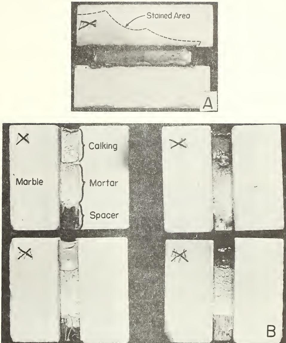
Fig. 1. Staining of marble and mortar caused by contact with Thiokol base calking compounds:
