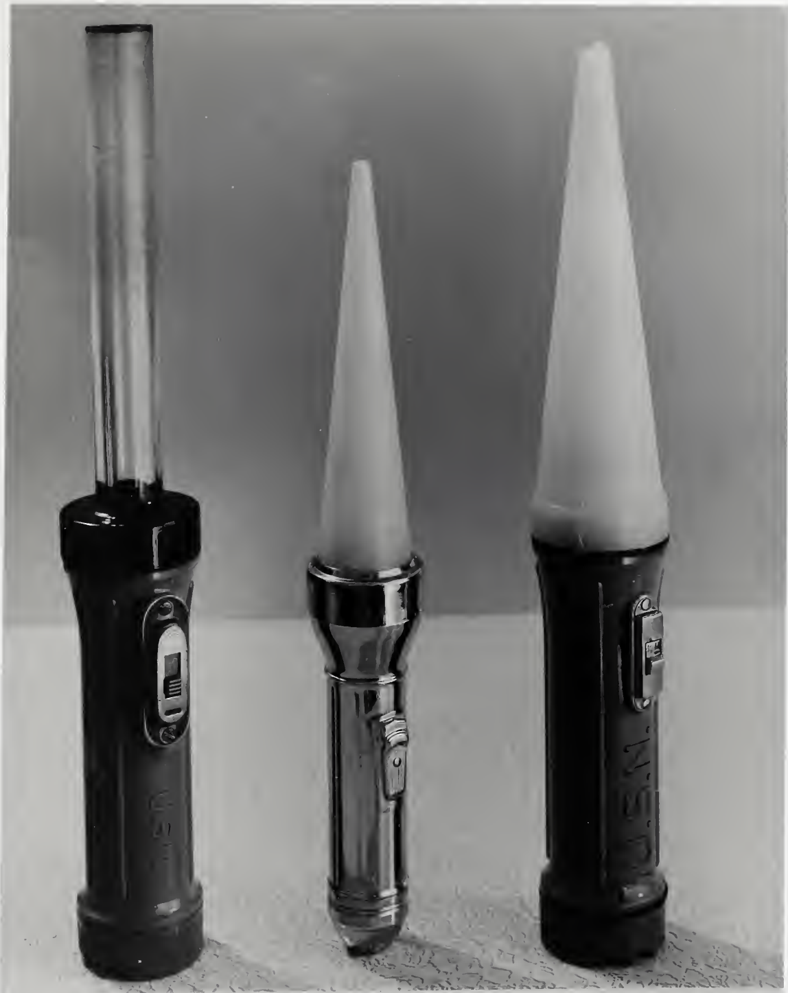
Taxi Guidance Wands: A. Present model B. N.B.S. C-size cell model C. Polyethylene cone on Navy flashlight
