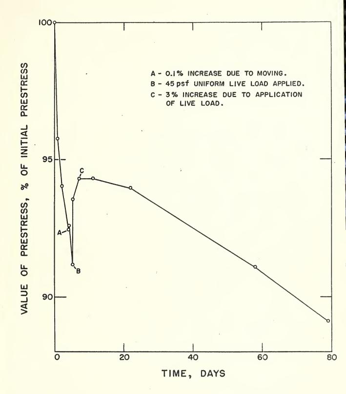
FIG. 4 VARIATION OF PRESTRESS WITH LOAD AND TIME.
