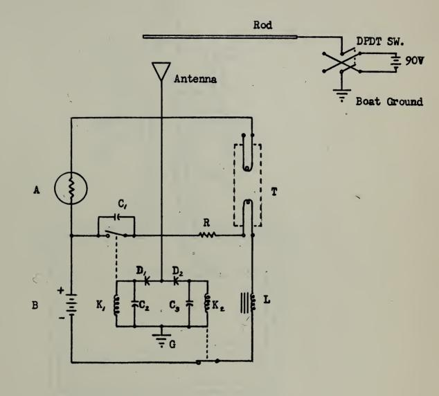
A Amperite, Type ITF15 B Batteries, 90V C, Capacitor, .01µf 1 C<sub>2</sub>,C<sub>3</sub> Capacitors, 50µf, 50WVDC D, D<sub>2</sub> Selenium Rectifier, 75ma., 20 Volts RMS, Federal Catalogue 1001 G Buoy Ground K, N.O. "On" Relay, Potter & Brumfield Type PW5LS, 10KA, 24V N.C. "Off" Relay K<sub>2</sub> 11 Ħ 11 11 H. Inductor, 1 HY, 20-24 A L Resistor 300 . , 10 Watt R T Fluorescent Lamp, 6 Watt
