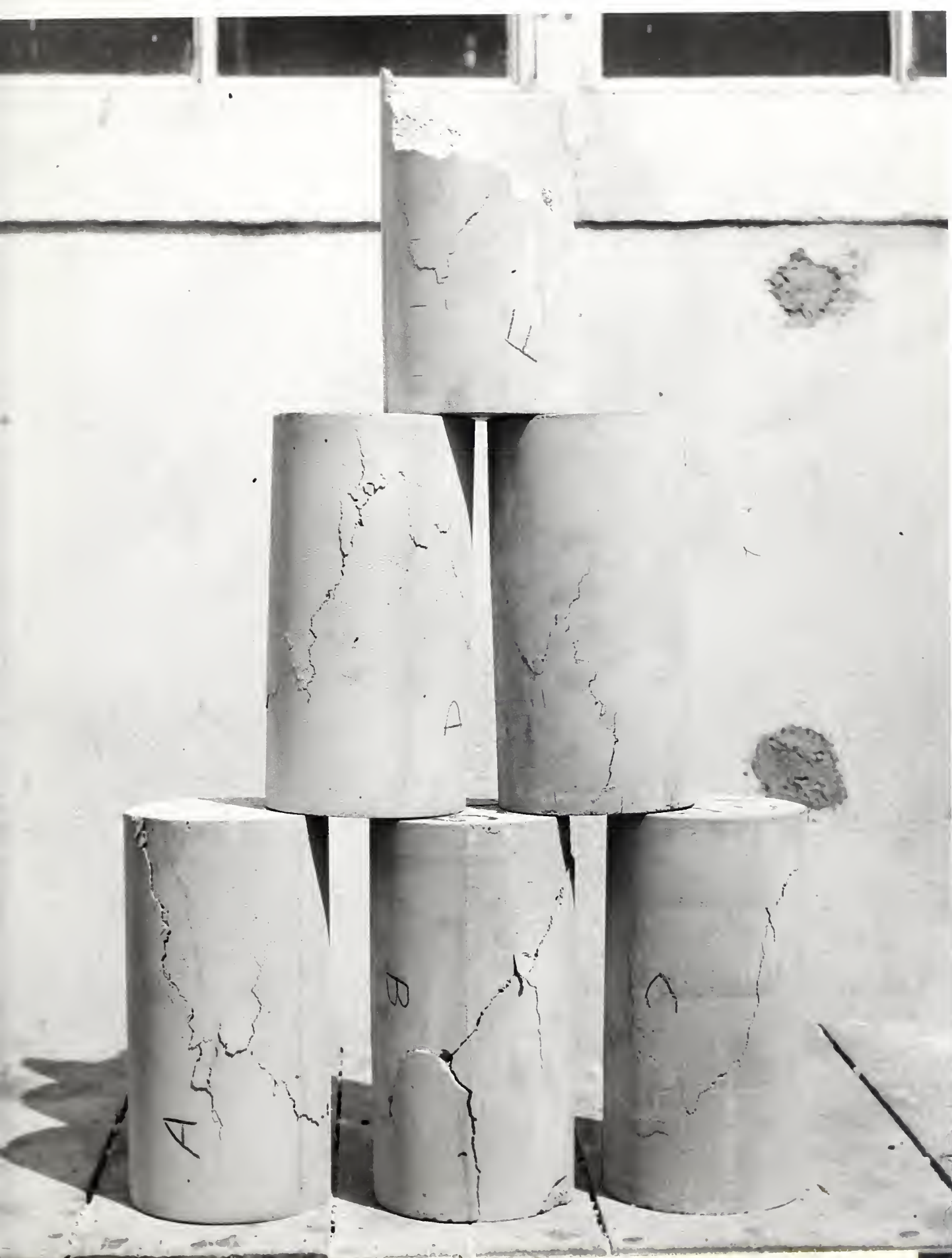
Fig. 2. Complete failure of cellular concrete 6- by 12-in. cylinders.
