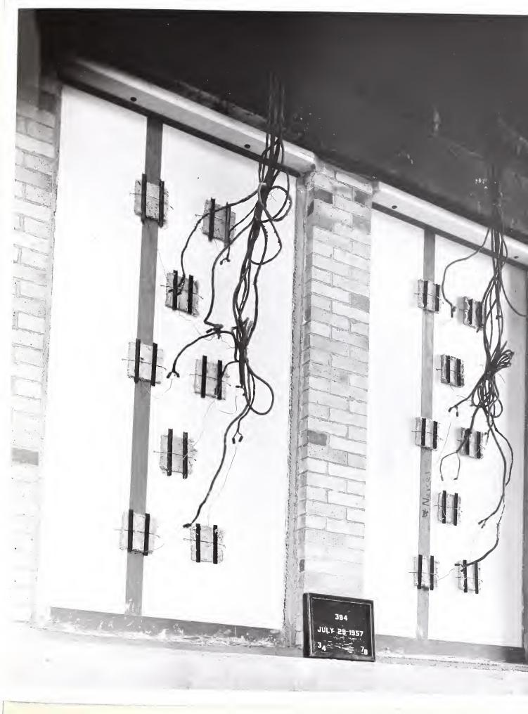
Fig. 6. Unexposed surfaces of specimens at end of test 394
