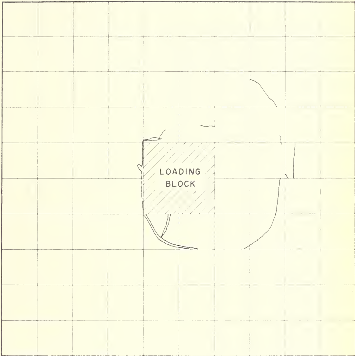
TOP VIEW AFTER FAILURE (BOTTOM SURFACE INTACT)
