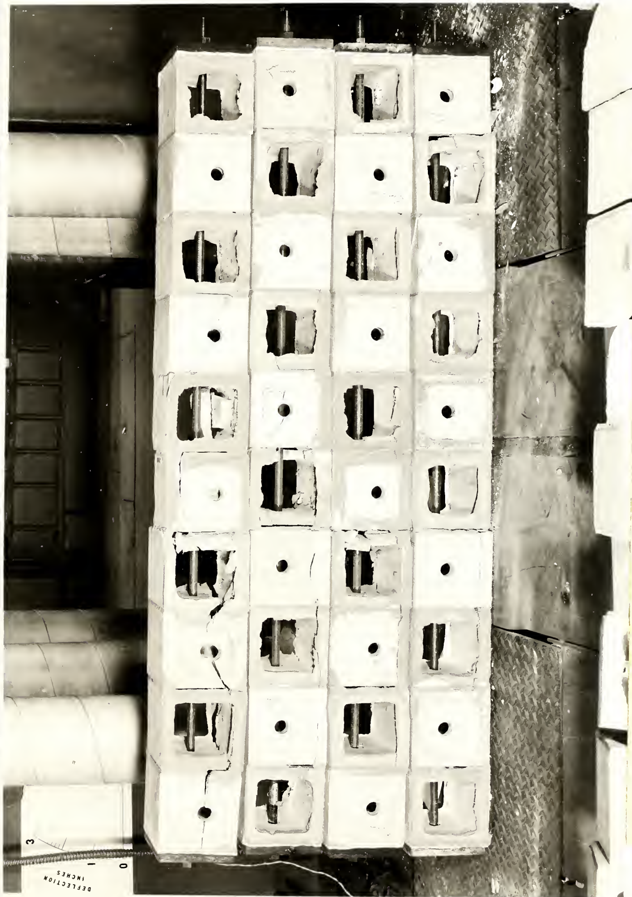
Fig. 25. View of sections through Slab No. 9.
