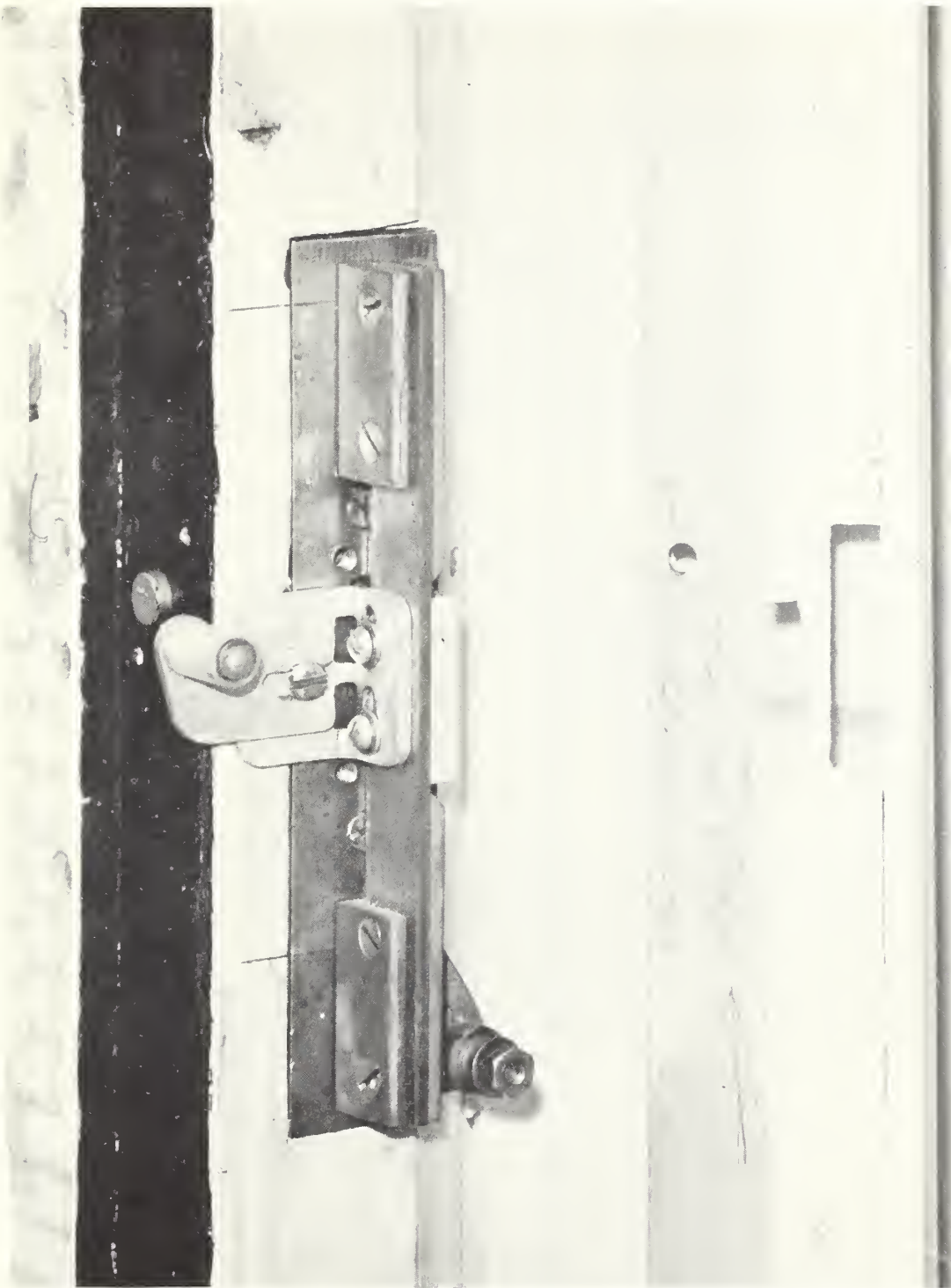
FIGURE 22. Assembly in door jamb to which door keepers for different release devices were attached (molding has been moved to right to show assembly).
