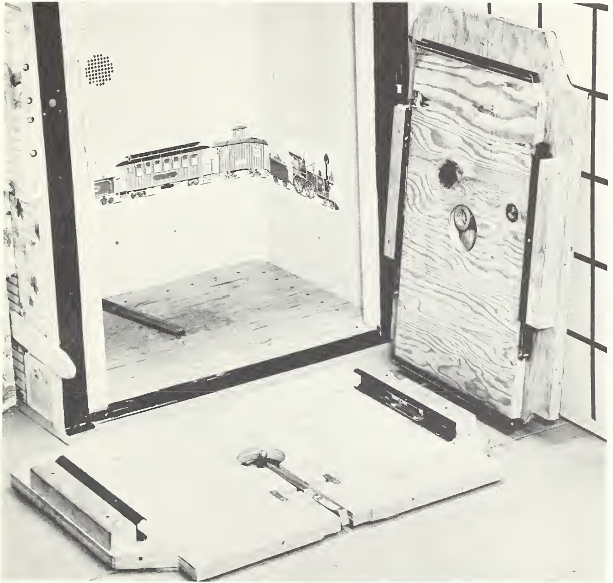
FIGURE 25. Construction detail of movable floor panel, illustrating ball-and-cone assembly and ball-bearing tracks.
