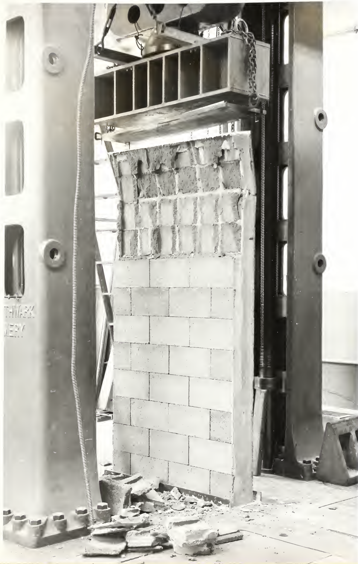
Fig. 8 - Compression Wall No. 3 after failure.
