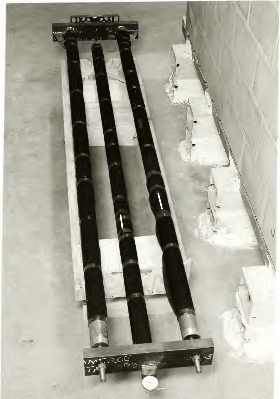
Fig. 9 - Horizontal comparator used in measuring length changes of shrinkage specimens.
