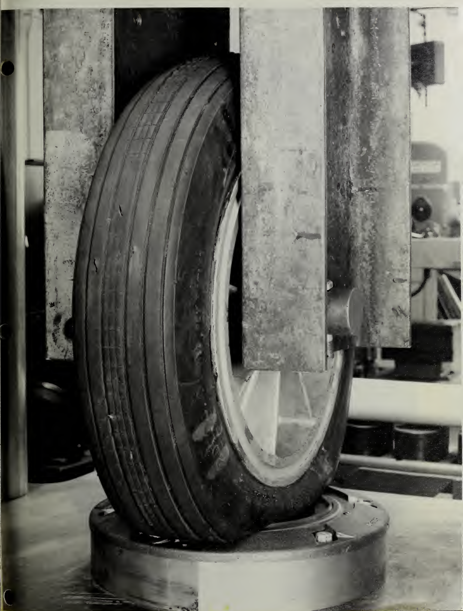
Figure 2. The light head assembly sustaining a load of 9,100 lb applied through a 20x4.4 aircraft tire.
