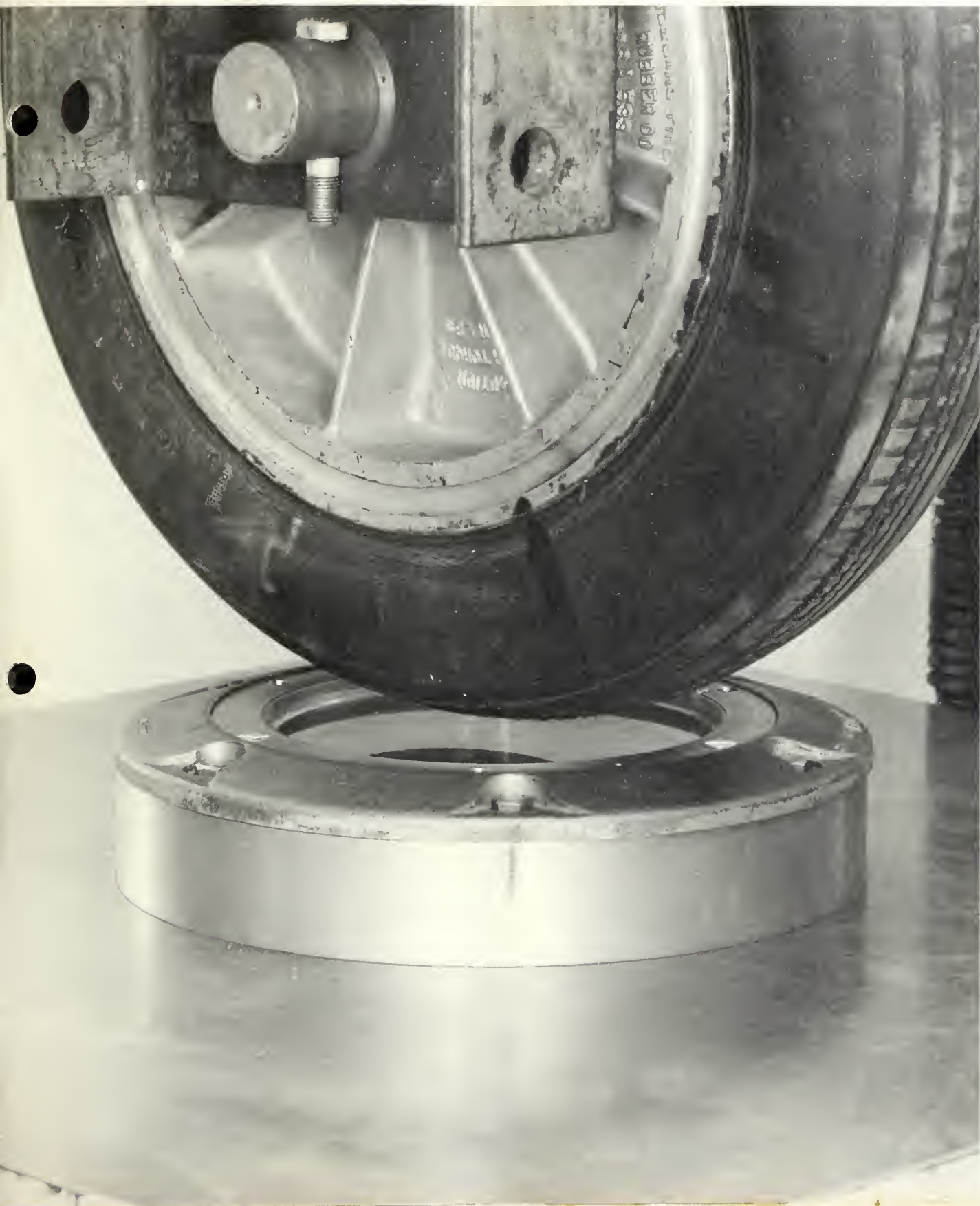
Laboratory set-up for compression test of sample A-3/4" with a 20x4.4 aircraft tire.
