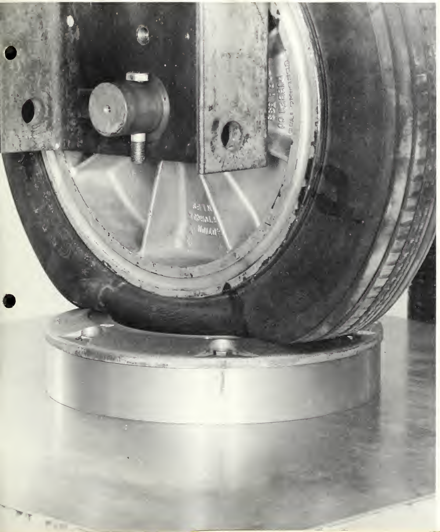
Sample A-3/4" with a load of 9,000 lb applied through the 20x4.4 tire.
