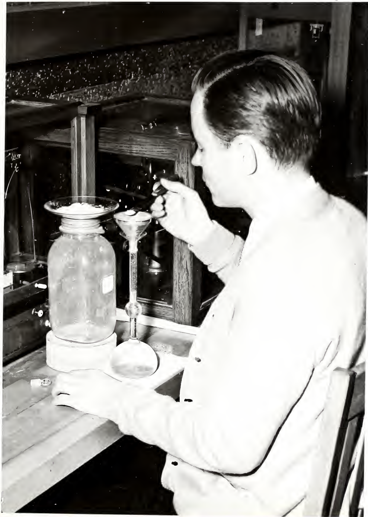
Fig. 8. True density determination showing operator filling a Le Chatelier flask with powdered sample under test.
