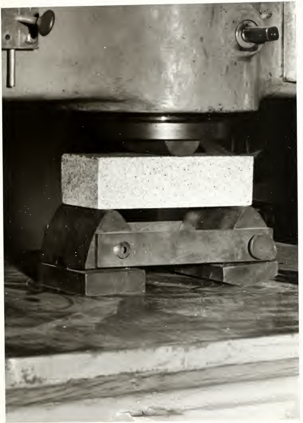
Fig. 3. Device for measuring flexural strength showing brick shaped specimen in position for test.
